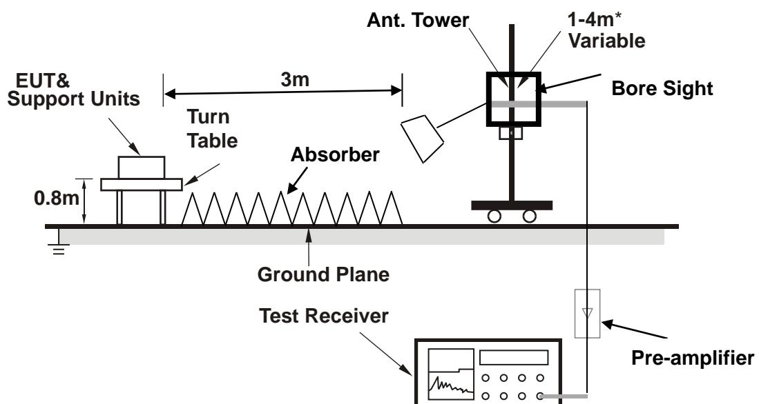
**Note:** Above 1G is a directional antenna depends on the EUT height and the antenna 3dB beamwidth both, refer to section 7.3 of CISPR 16-2-3.
