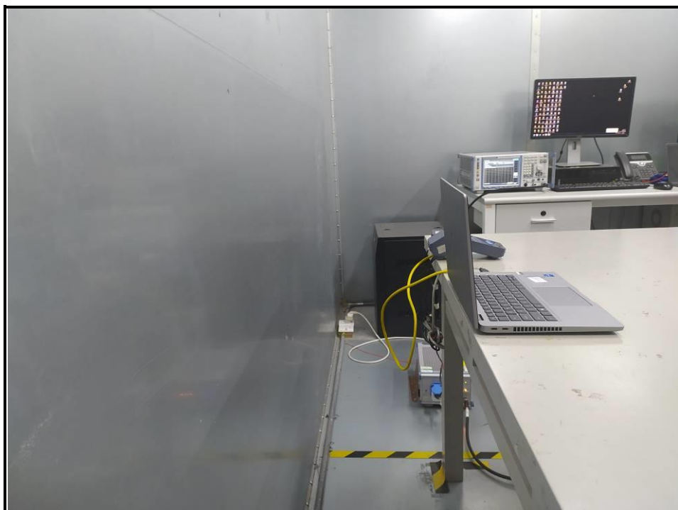
Fig. 4 Power line conducted emission setup photo
