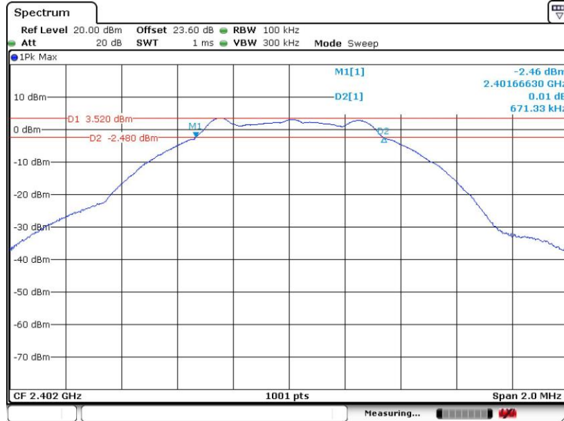
6 dB Bandwidth Plot on Channel 00
