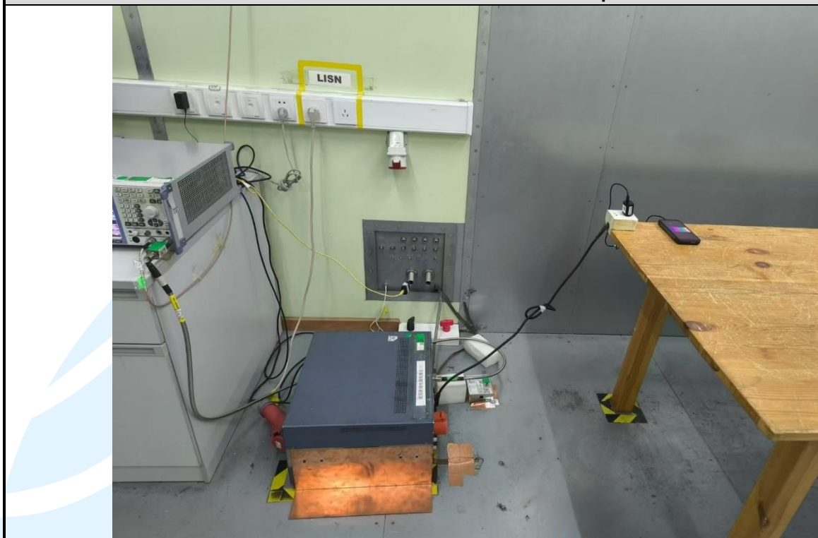
Conducted Emission Test Setup
