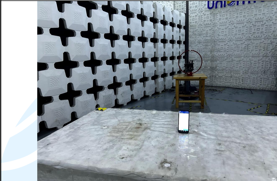
Radiated emission Test Setup (Below 30 MHz)
