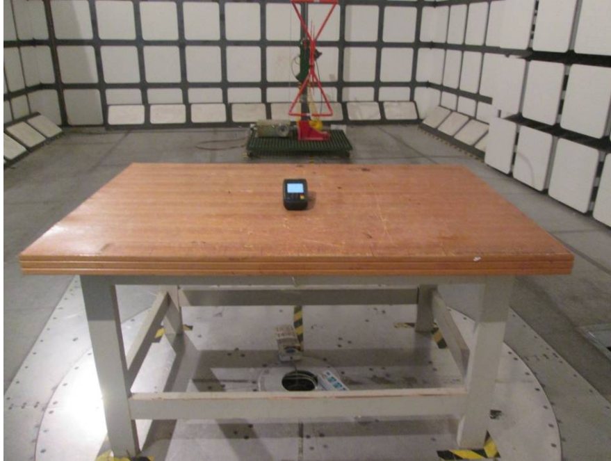
Radiated Emissions View (Below 1 GHz)
