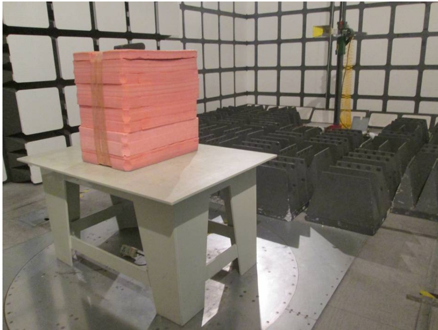
Radiated Emissions View (Above 1 GHz)
