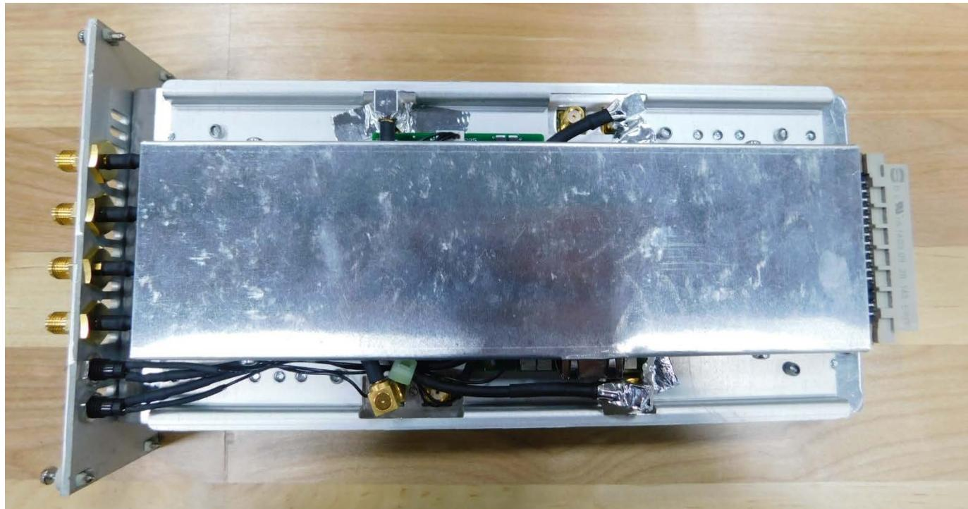
1.2 Bottom view with Mechanical Plate Cover
