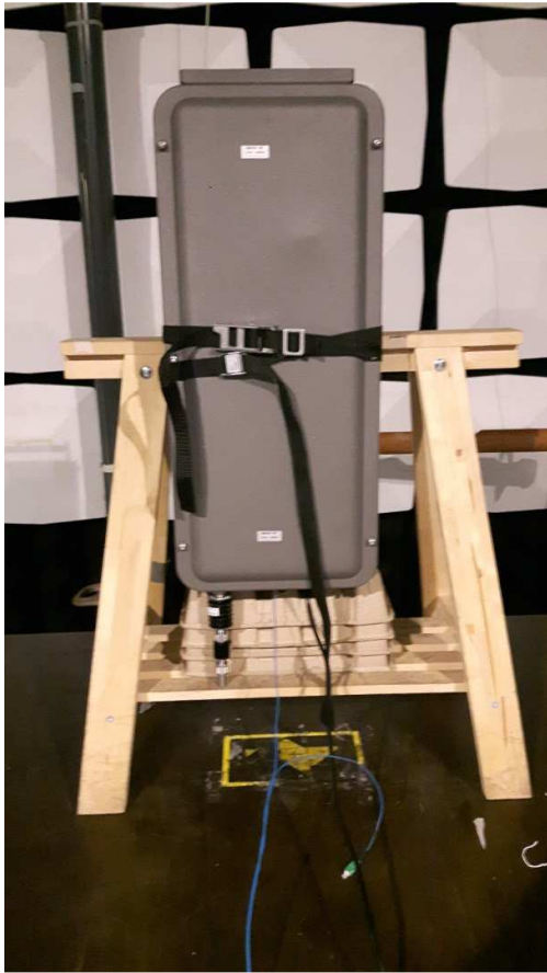
Test set up radiated emission 30 MHz – 1GHz
