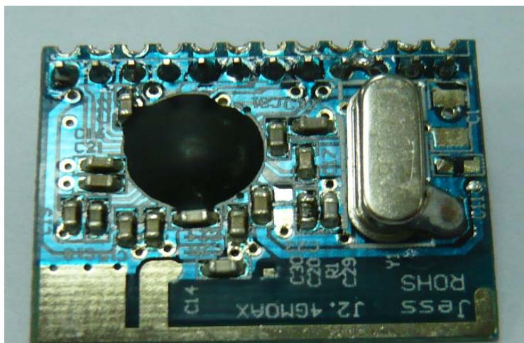
Size : 25.4mm x 21.0mm, connector pad pitch : 2mm
