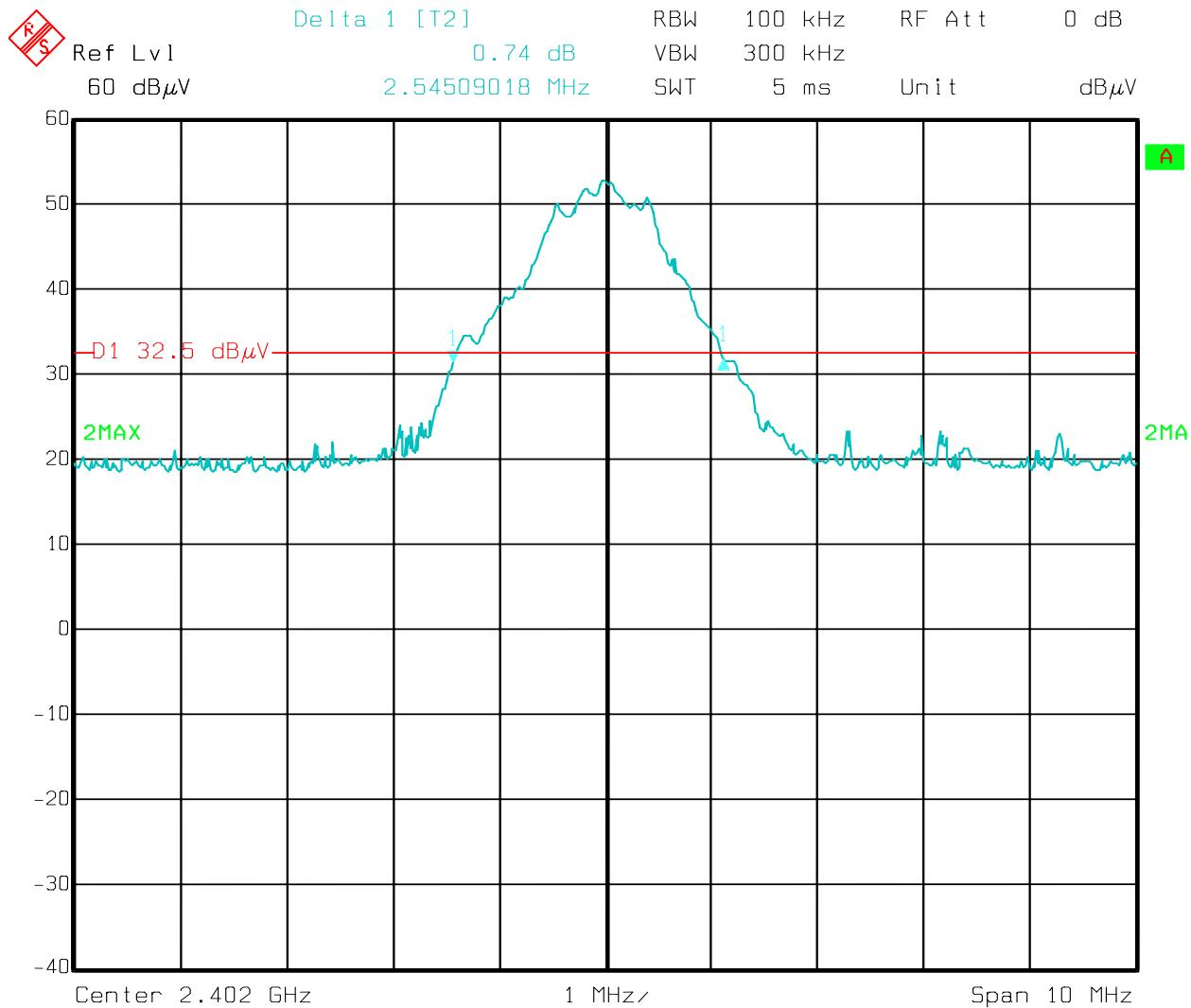
**LOW Channel - Measured Occupied Bandwidth is 2.54MHz.**
