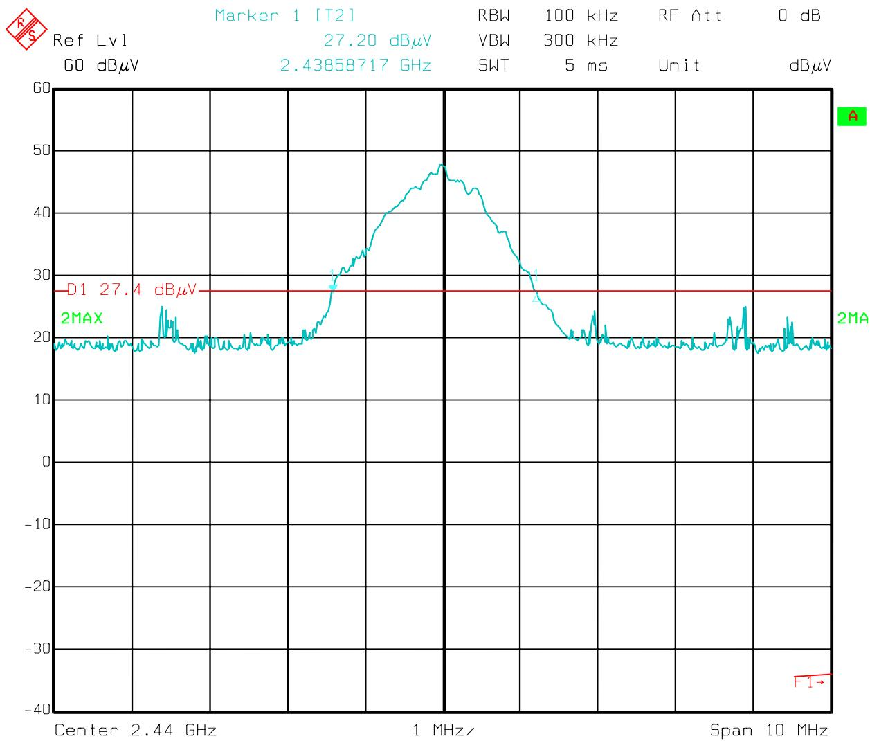
**MID Channel - Measured Occupied Bandwidth is 2.44 MHz.**
