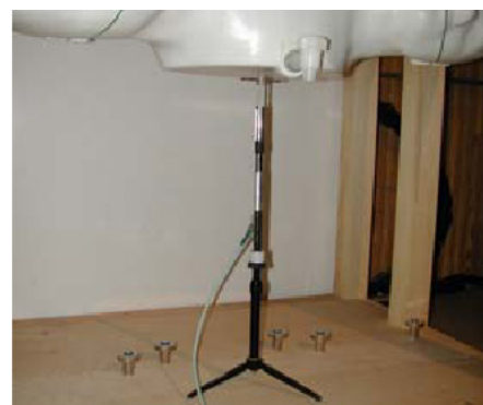
Figure 12.1 Dipole Validation Test Setup
