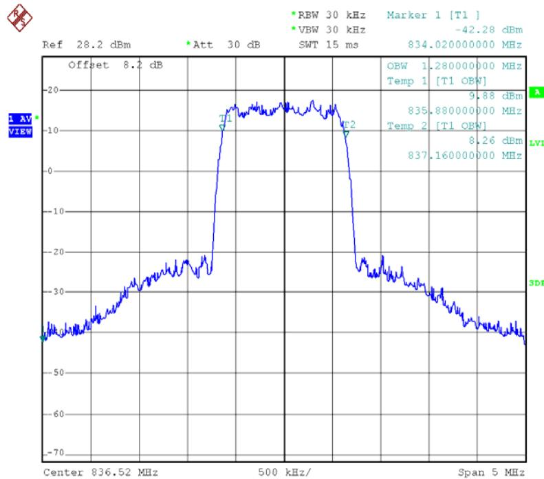
**- Occupied Bandwidth CDMA Mode ch.384 for 1xEV-DO**
