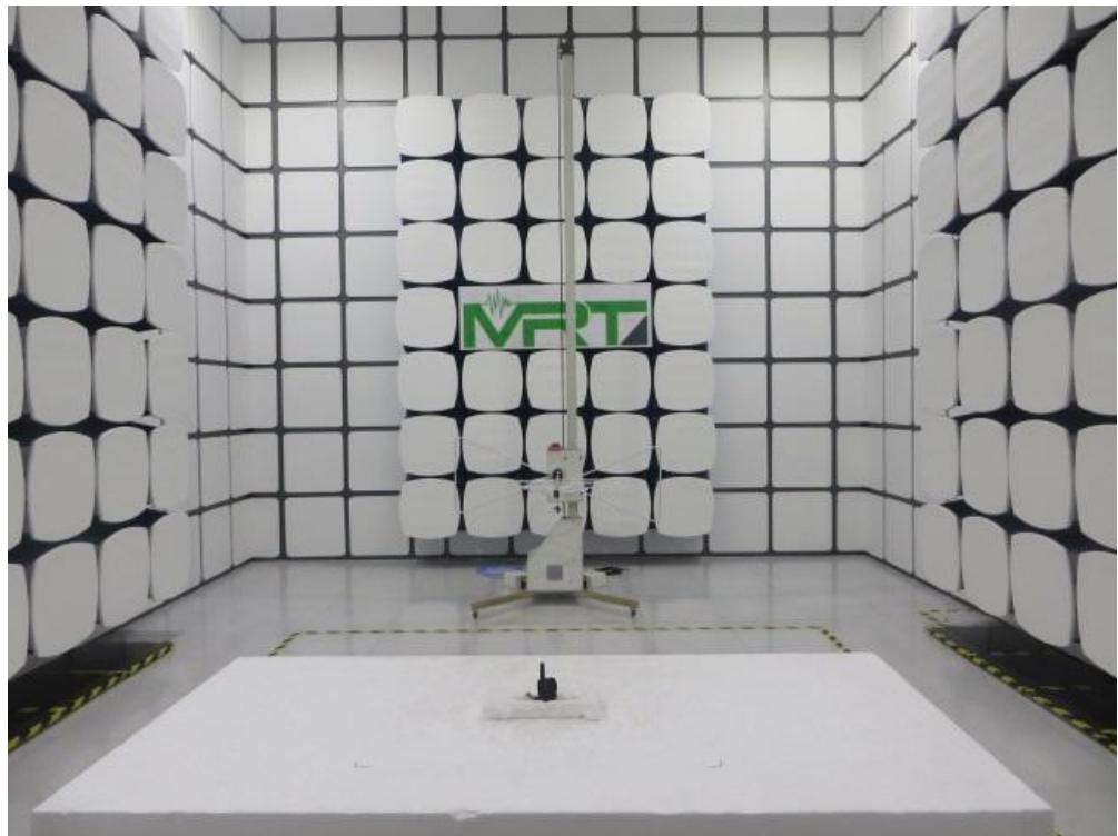
Description: Radiated disturbance Test Setup for Above 1GHz
