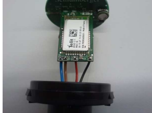
Diver-DXT with radio board (two sides)
