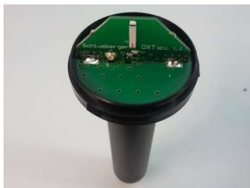
Diver-DXT with radio board, cap (with o-ring) and lithium battery
