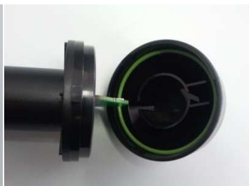
Diver-DXT with radio board, cap (with o-ring) and lithium battery
