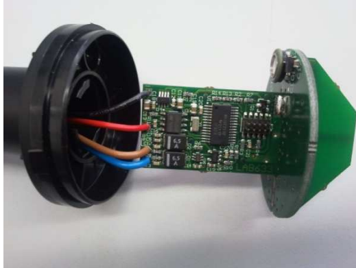
Diver-DXT with radio board (two sides)
