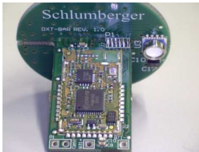
Diver-DXT radio shielding removed
