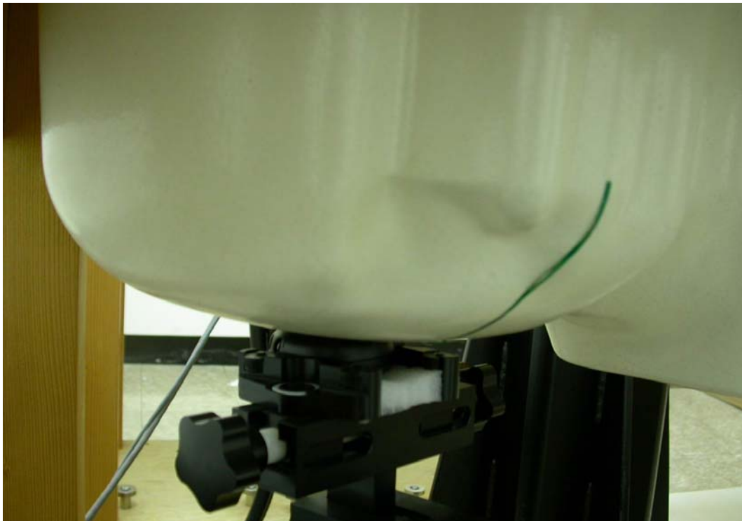
Measurement Position of Right-Cheek (RC) with Handset
