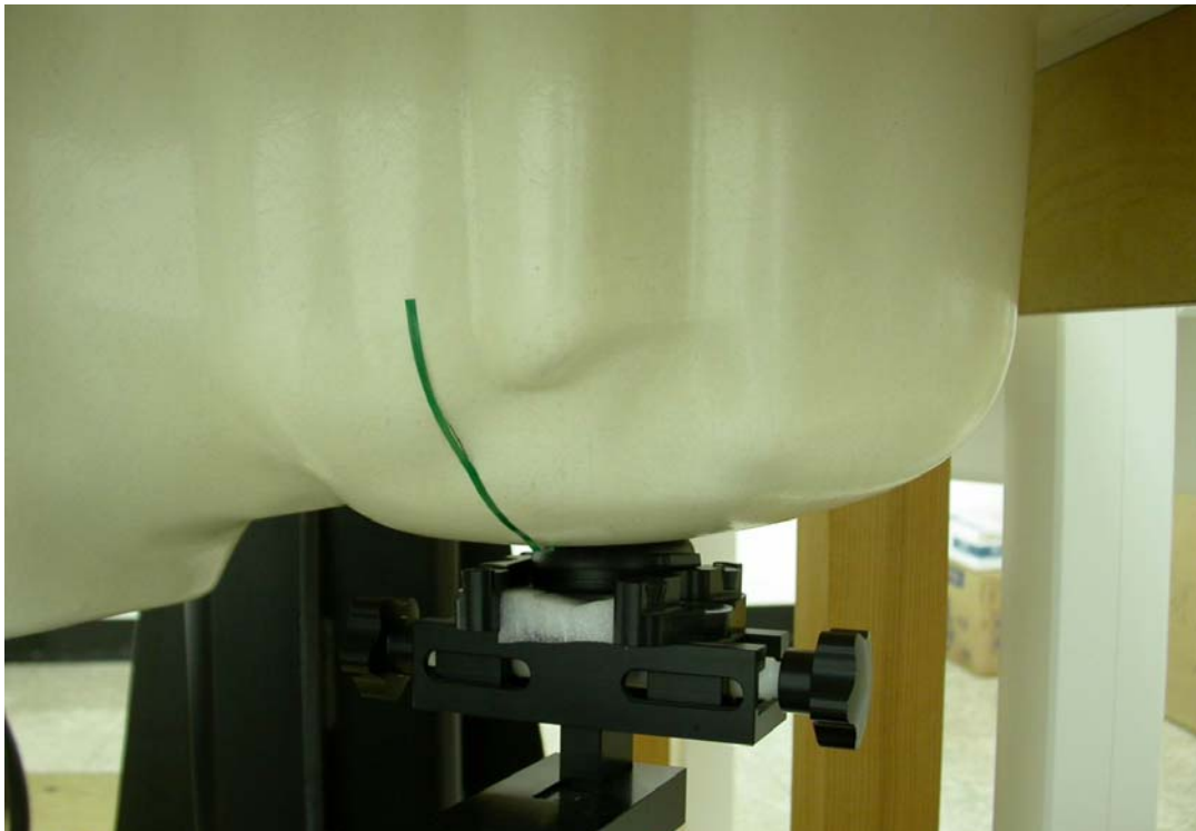
Measurement Position of Left-Cheek (LC) with Handset
