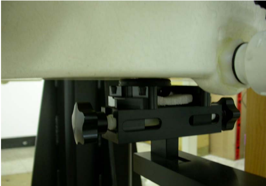
Measurement Position of Body Rear-UP with Handset
