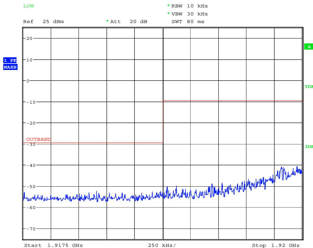
Out-of-band Unwanted Emissions: CH F<sub>L</sub>.
