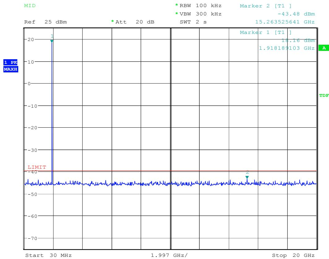
c) CH F<sub>H</sub>Out-of-band Unwanted Emissions (below 1GHz): CH F<sub>H</sub>
