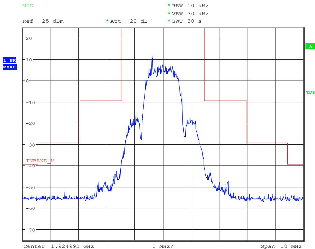
**In-band Unwanted Emissions: CH FH**
