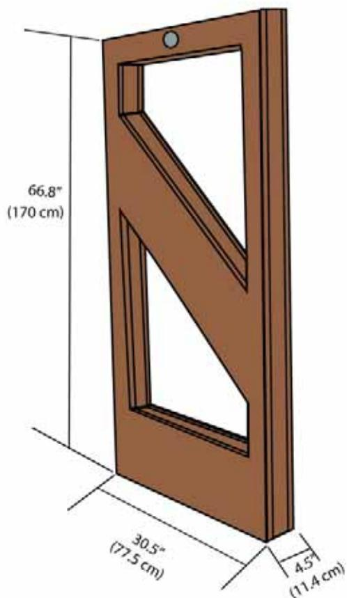
Figure 2: Antenna outside dimensions
