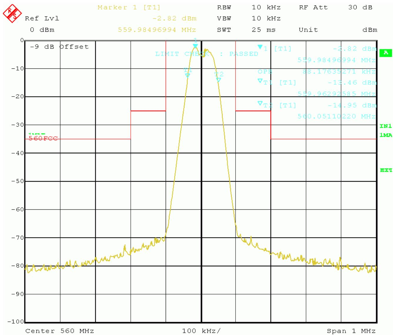
Measured 99% power Bandwidth: 88,2kHz
