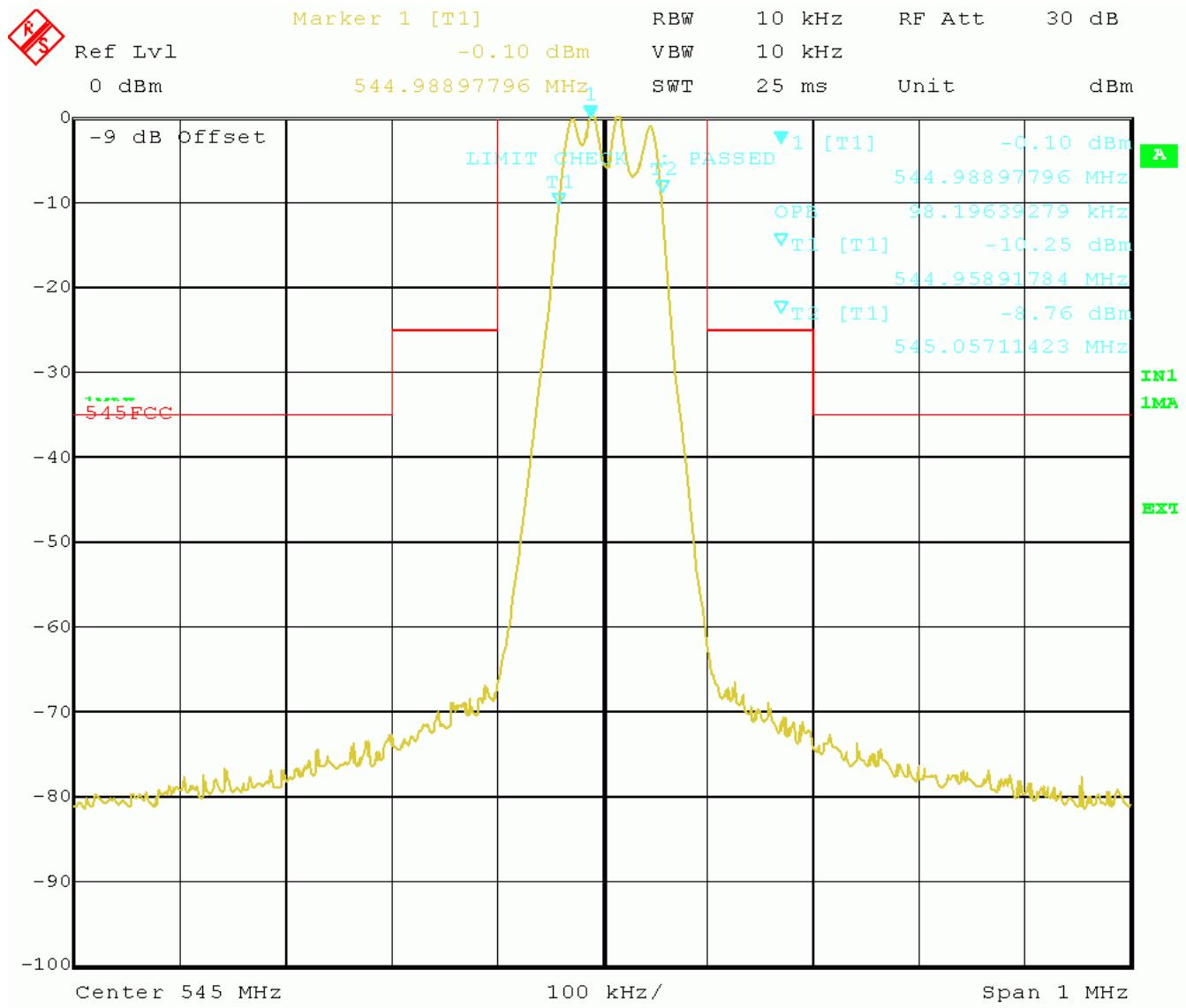
Measured 99% power Bandwidth: 98,2kHz
