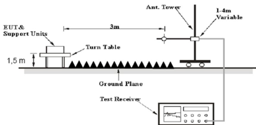
The radiated emission tests were performed in the 3 meters chamber test site, using the setup accordance with the ANSI C63.10-2013. The specification used was the FCC 15.209, and FCC 15.247 limits.
