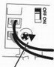
Adjust the potentiometer clockwise
