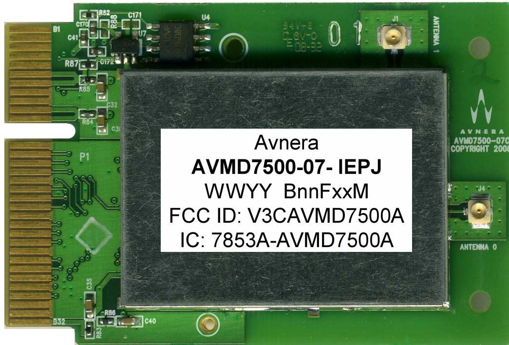
Note that the fields on Line 2 ("MMYY BnnFxxM") will be used for date code and production tracking information, and will change with every manufacturing lot.
