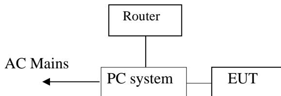
7.1.2. Semi-anechoic Chamber Test Setup Diagram
