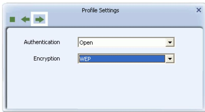
**B.** In the 'WEP Key' field, type the same WEP key as that configured on the AP or wireless router to which you are connecting, and ensure that 'Default Tx Key' and 'Key Format' settings are also the same. Click the right arrow to save your settings and connect to the network.
