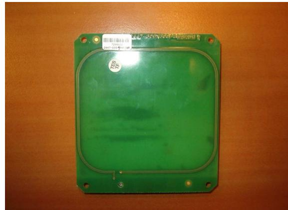
Each antenna is connected to the motherboard with a coaxial cable on HFL or UFL connectors
