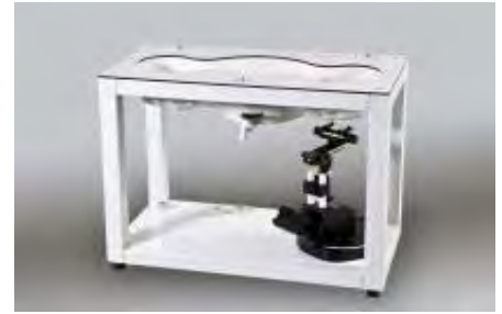
Figure E.5.1 SAM Twin Phantom
