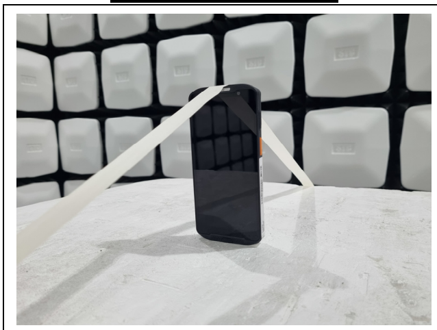
EUT Position: Y-axis
