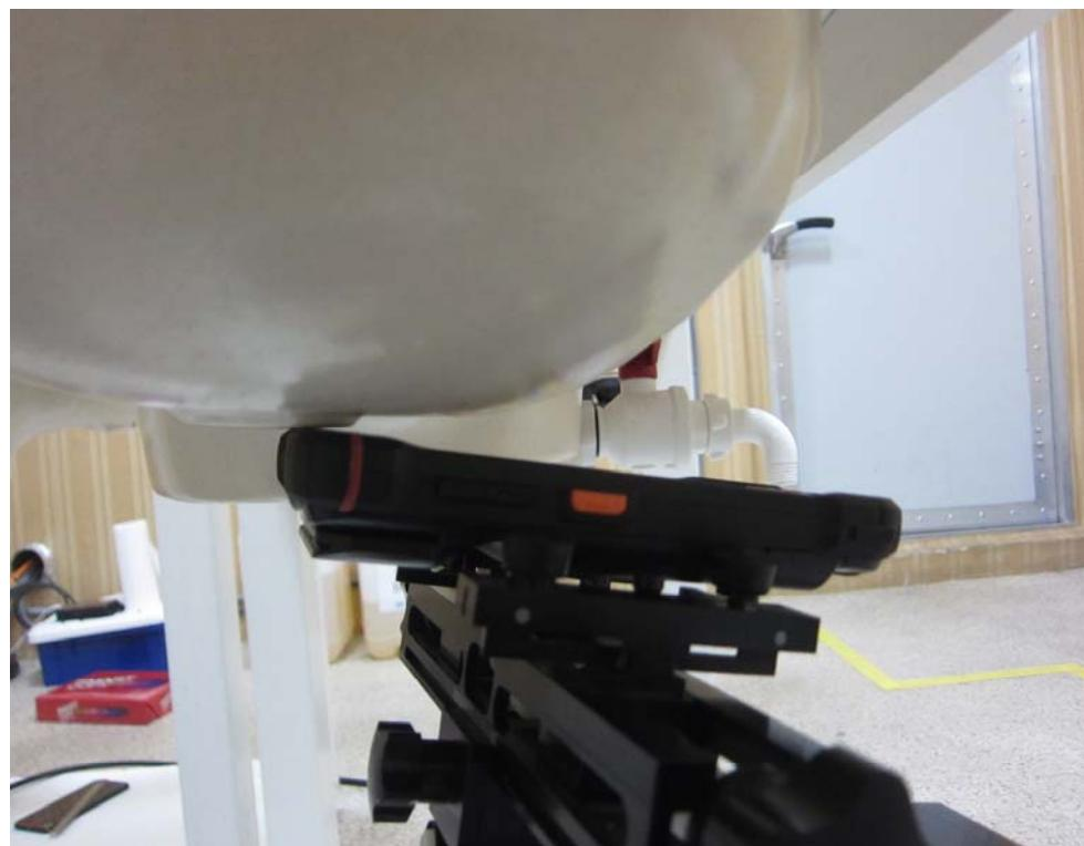
**■ Test Setup Photo (Head SAR Test Photo)**
