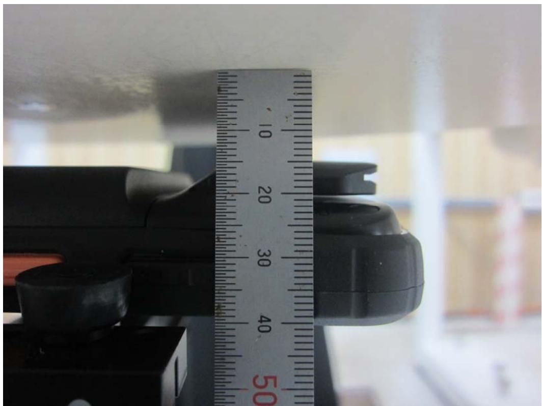
**■ Test Setup Photo (Phablet SAR Test Photo)**
