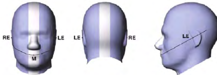
Figure 4.2 Front, back and side view SAM Twin Phantom
