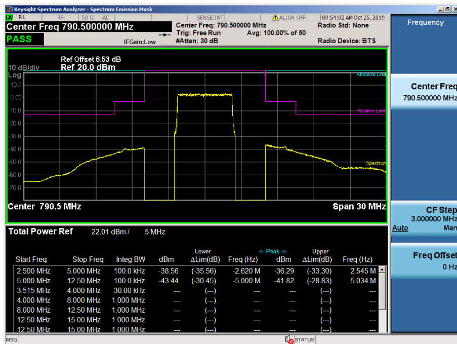
LTE Band 14 / 5MHz / QPSK - RB Size/Offset (25/0) - Low Channel
