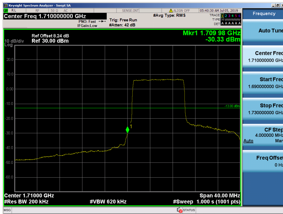
LTE Band 4 / 20MHz / QPSK - RB Size/Offset (50/0)
