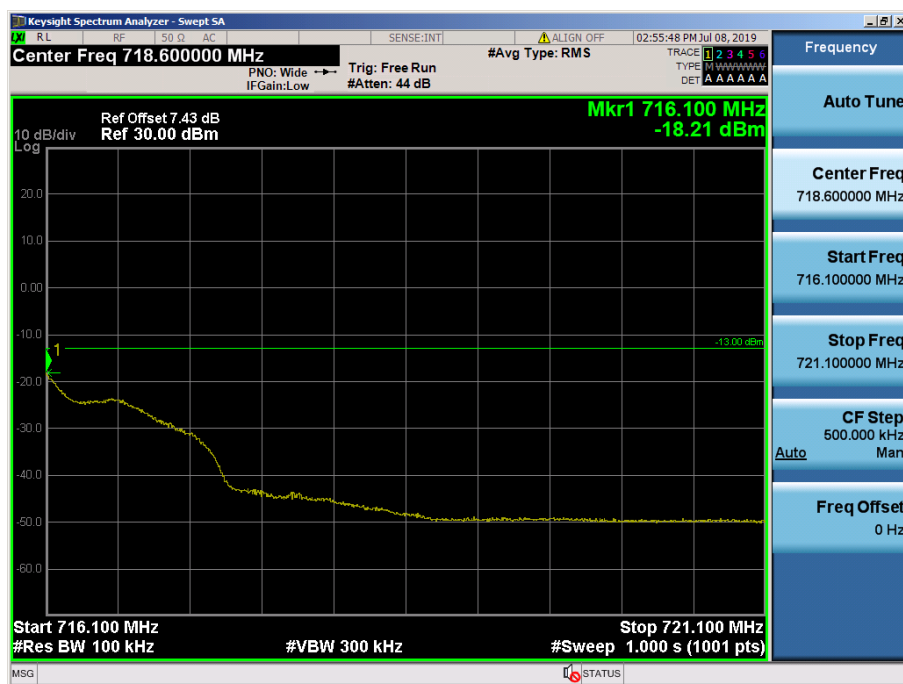
LTE Band 12 / 3MHz / QPSK - RB Size/Offset (8/7)
