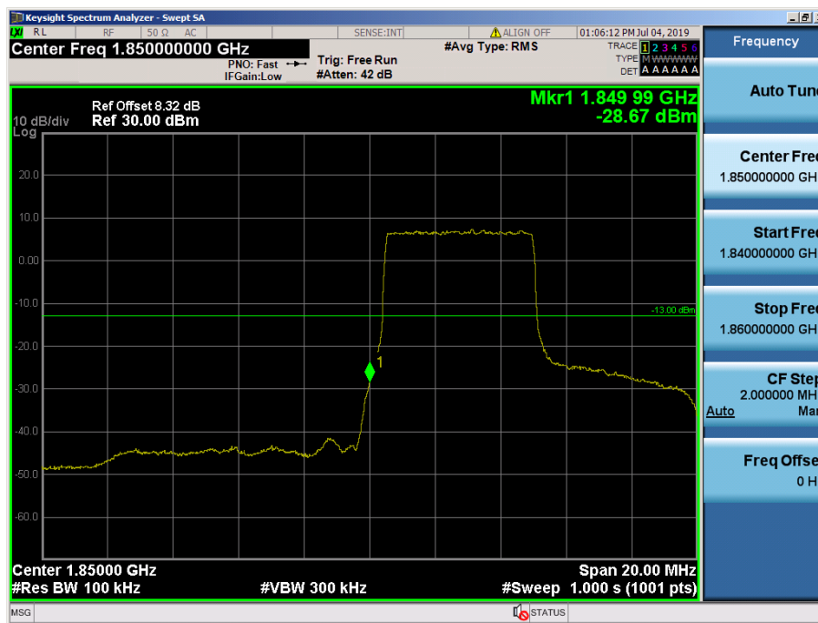
LTE Band 25 / 10MHz / QPSK - RB Size/Offset (25/0)
