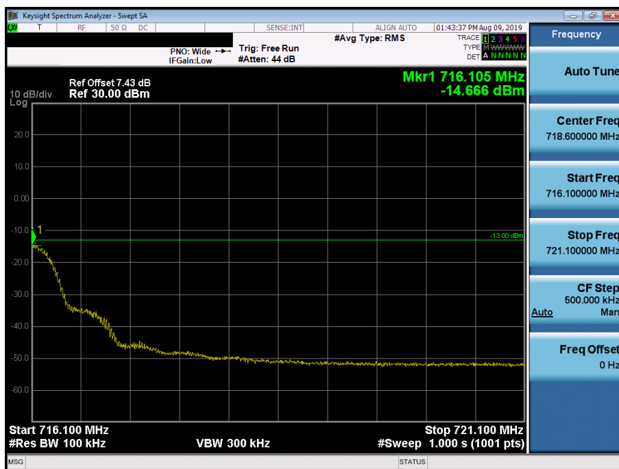
LTE Band 12 / 1.4MHz / QPSK - RB Size/Offset (3/3)
