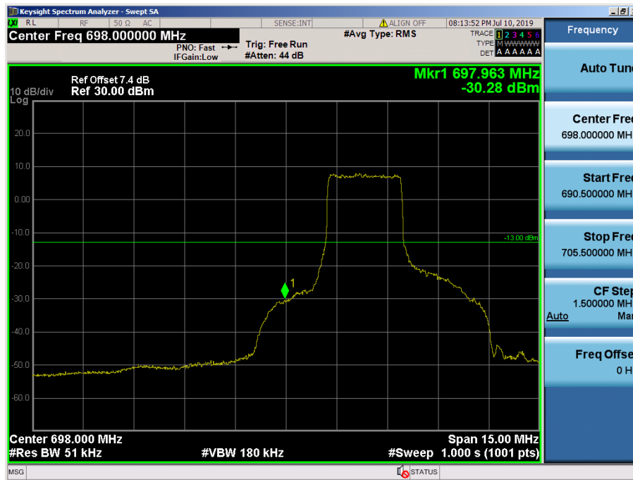
LTE Band 12, 17 / 5MHz / QPSK - RB Size/Offset (12/0)
