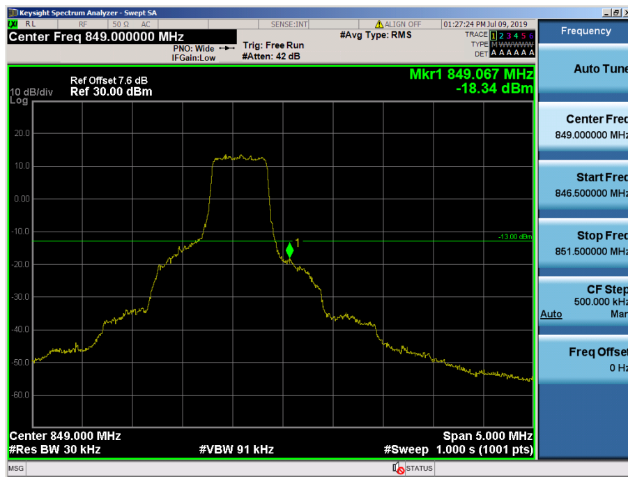
LTE Band 26 / 1.4MHz / QPSK - RB Size/Offset (3/3)
