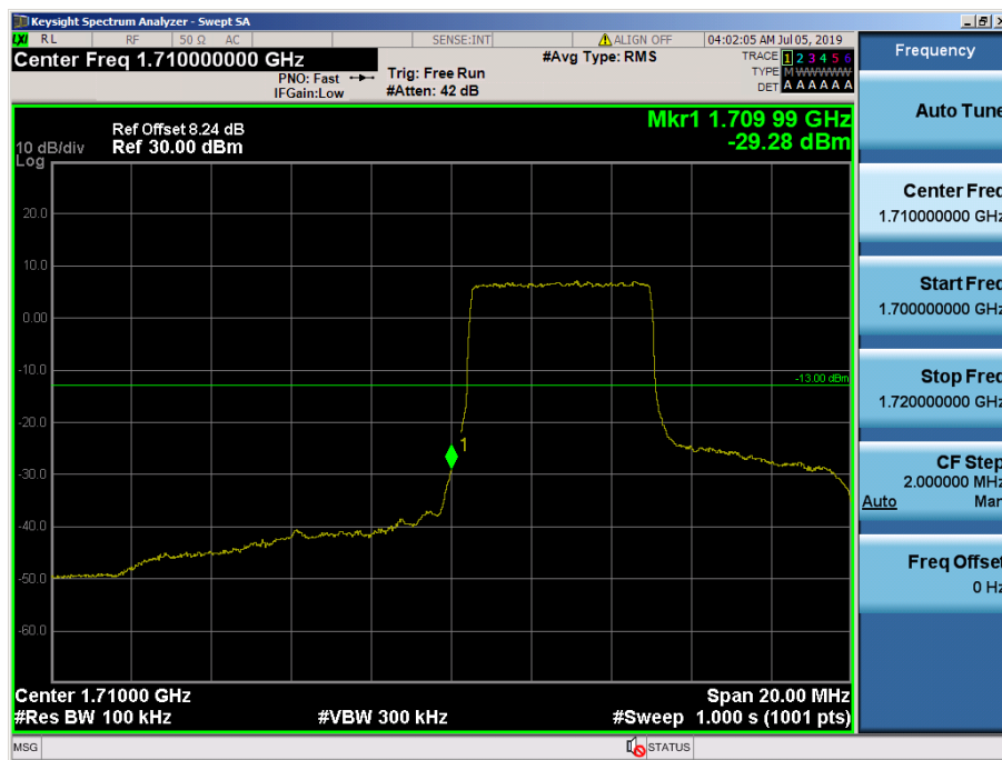
LTE Band 4 / 10MHz / QPSK - RB Size/Offset (25/0)
