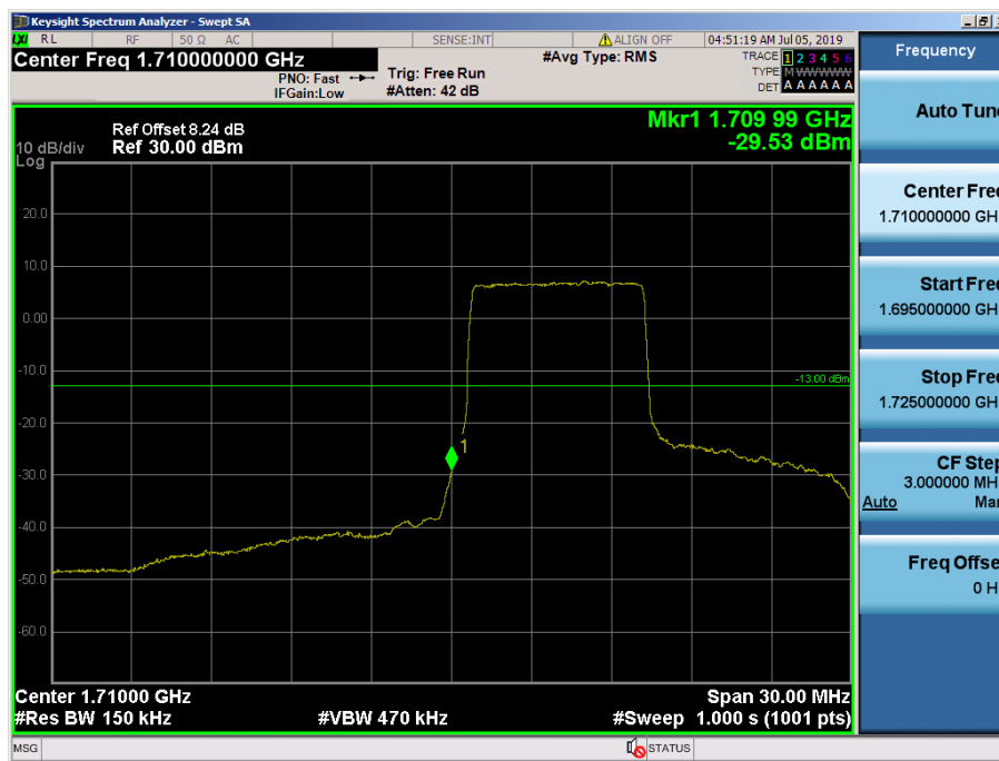
LTE Band 4 / 15MHz / QPSK - RB Size/Offset (36/0)
