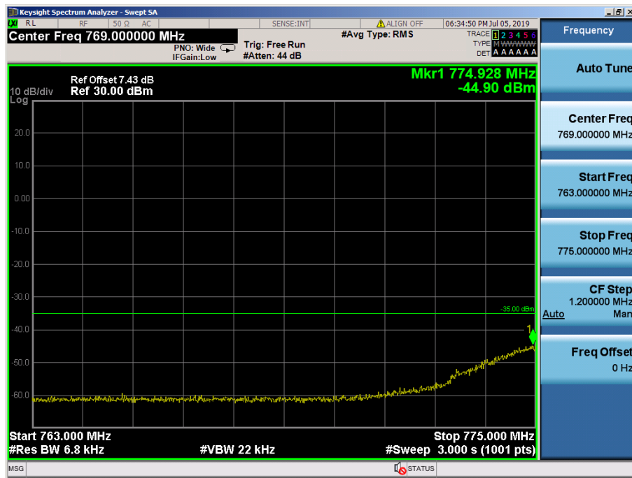
LTE Band 13 / 10MHz / QPSK - RB Size/Offset (25/0)
