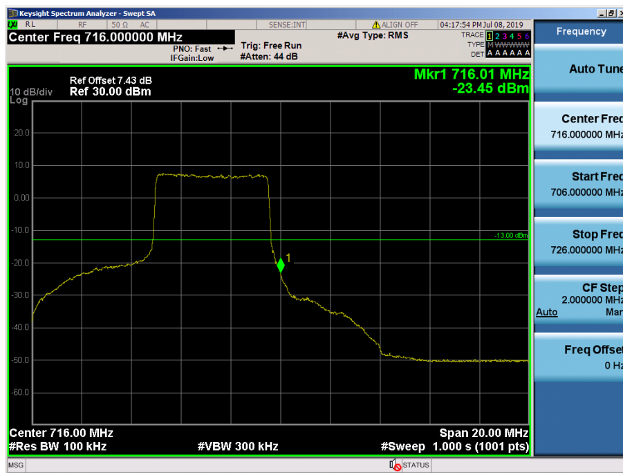
LTE Band 12, 17 / 10MHz / QPSK - RB Size/Offset (25/25)
