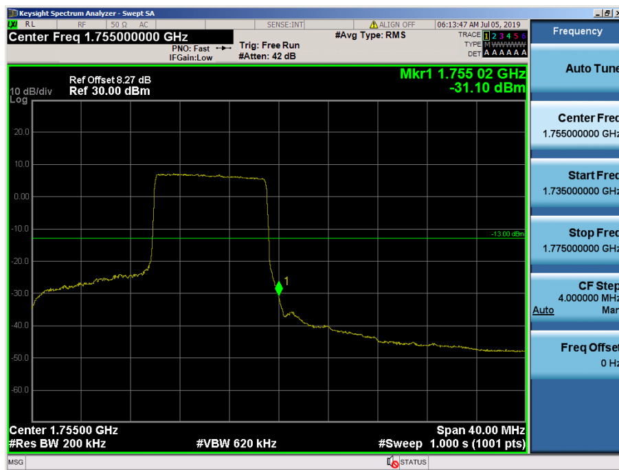
LTE Band 4 / 20MHz / QPSK - RB Size/Offset (50/50)
