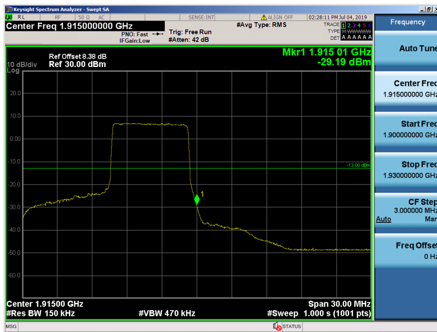
LTE Band 25 / 15MHz / QPSK - RB Size/Offset (36/39)
