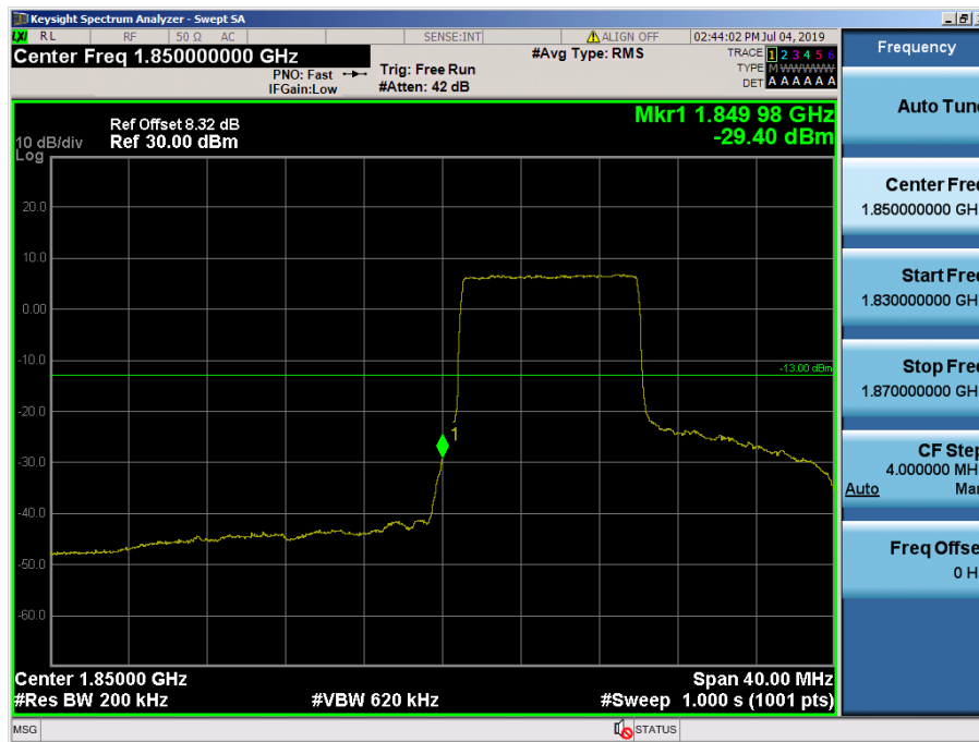
LTE Band 25 / 20MHz / QPSK - RB Size/Offset (50/0)
