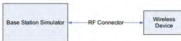
Figure 9.1 Power Measurement Setup
