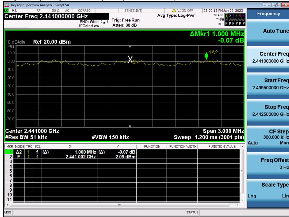
Carrier Frequency Separation (AFH) *Hopping mode : Enable& TM1 & 8DPSK*
