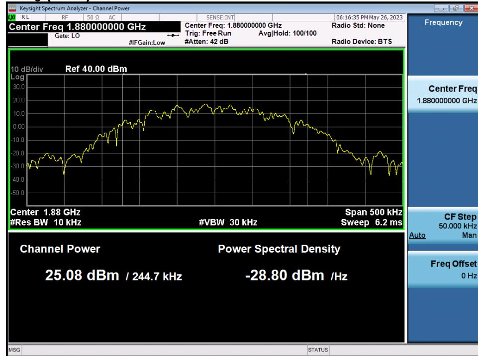
$$\text{PAPR (dB)} = \text{P}_{\text{Pk}} \text{ (dBm)} - \text{P}_{\text{Avg}} \text{ (dBm)} = 29.06 \text{ dBm} - 25.08 \text{ dBm} = 3.98 \text{ dB}$$
