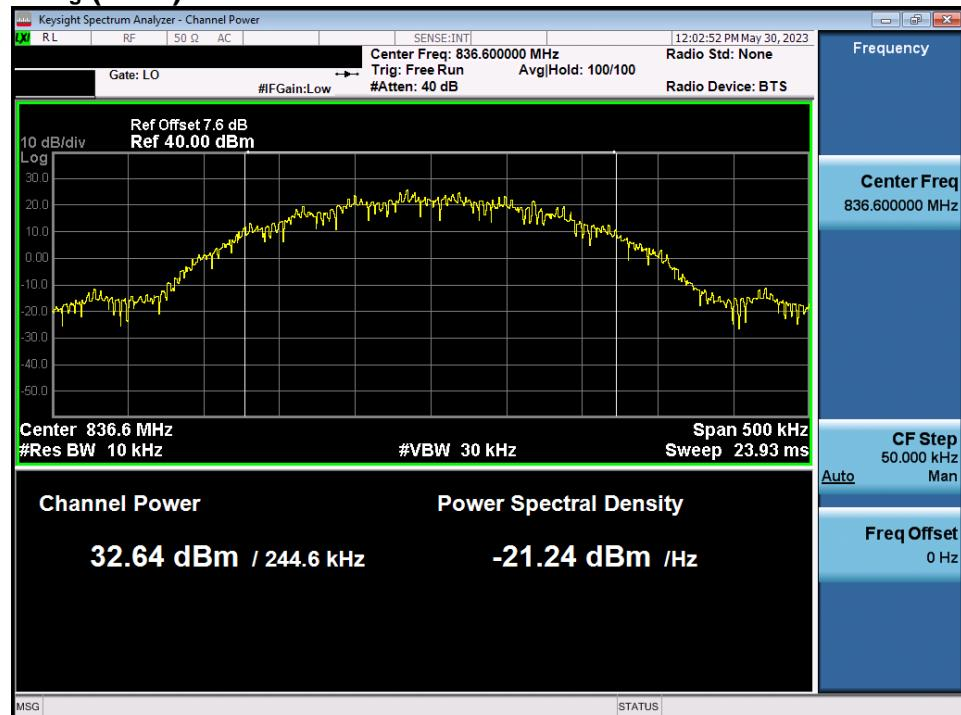
$$\text{PAPR (dB)} = \text{P}_{\text{Pk}} (\text{dBm}) - \text{P}_{\text{Avg}} (\text{dBm}) = 32.77 \text{ dBm} - 32.64 \text{ dBm} = 0.13 \text{ dB}$$
