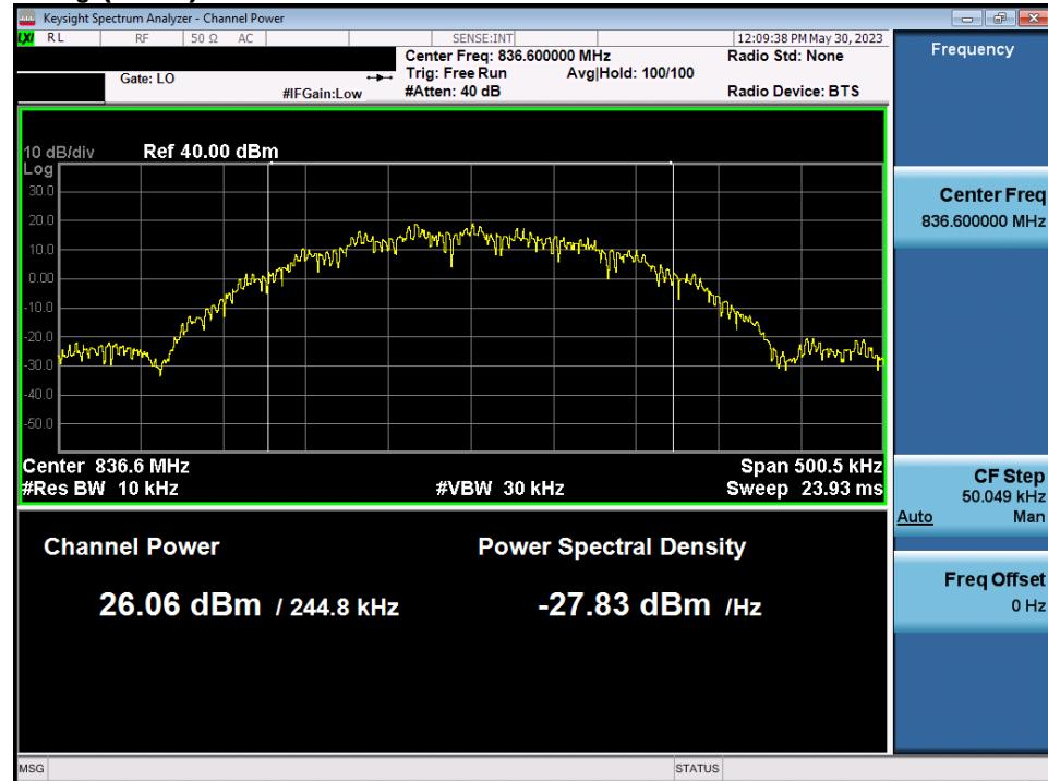
$$\text{PAPR (dB)} = \text{P}_{\text{Pk}} \text{ (dBm)} - \text{P}_{\text{Avg}} \text{ (dBm)} = 29.27 \text{ dBm} - 26.06 \text{ dBm} = 3.21 \text{ dB}$$
