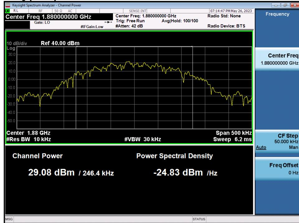
$$\text{PAPR (dB)} = \text{P}_{\text{Pk}} \text{ (dBm)} - \text{P}_{\text{Avg}} \text{ (dBm)} = 29.27 \text{ dBm} - 29.08 \text{ dBm} = 0.19 \text{ dB}$$
