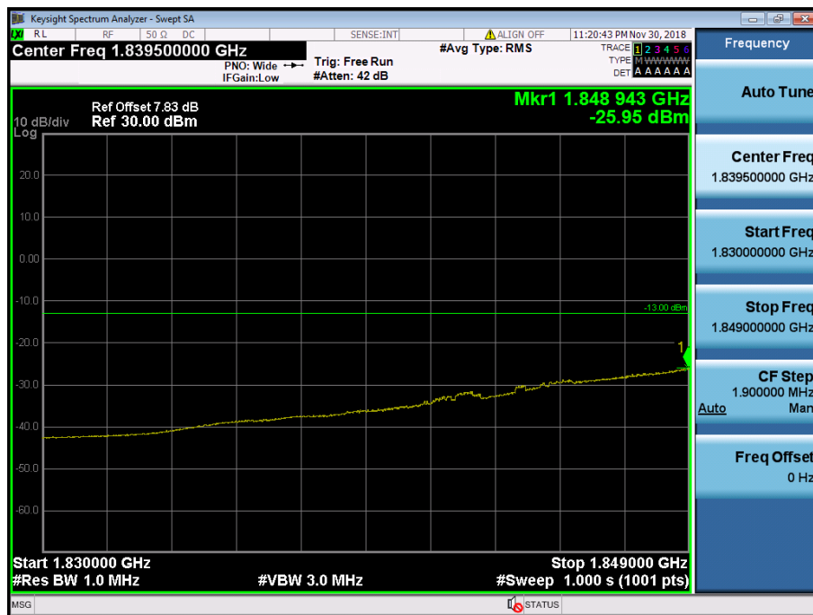
LTE Band 2 / 20MHz / QPSK - RB Size/Offset (50/0)
