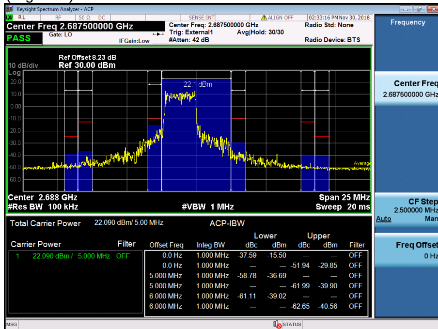
LTE Band 41 / 5MHz / QPSK - RB Size/Offset (12/0)
