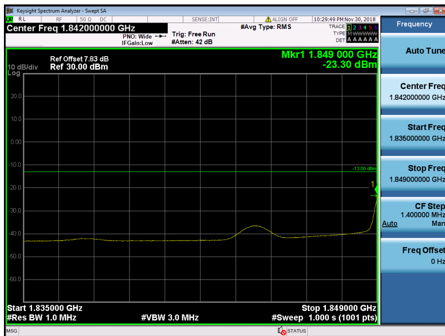
LTE Band 2 / 15MHz / QPSK - RB Size/Offset (1/0)
