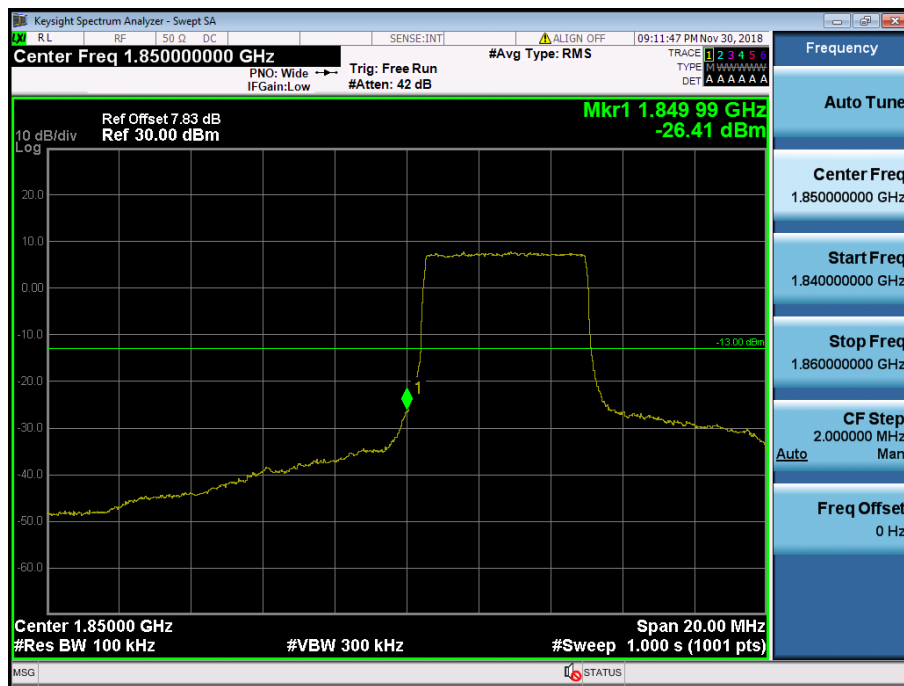
LTE Band 2 / 10MHz / QPSK - RB Size/Offset (25/0)
