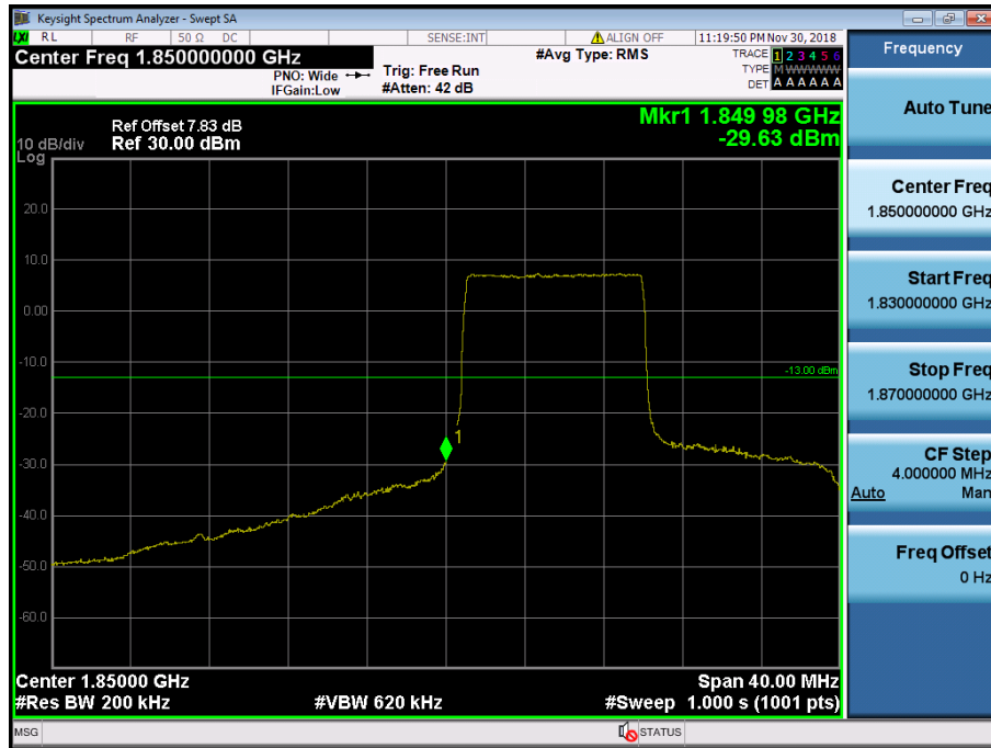
LTE Band 2 / 20MHz / QPSK - RB Size/Offset (50/0)
