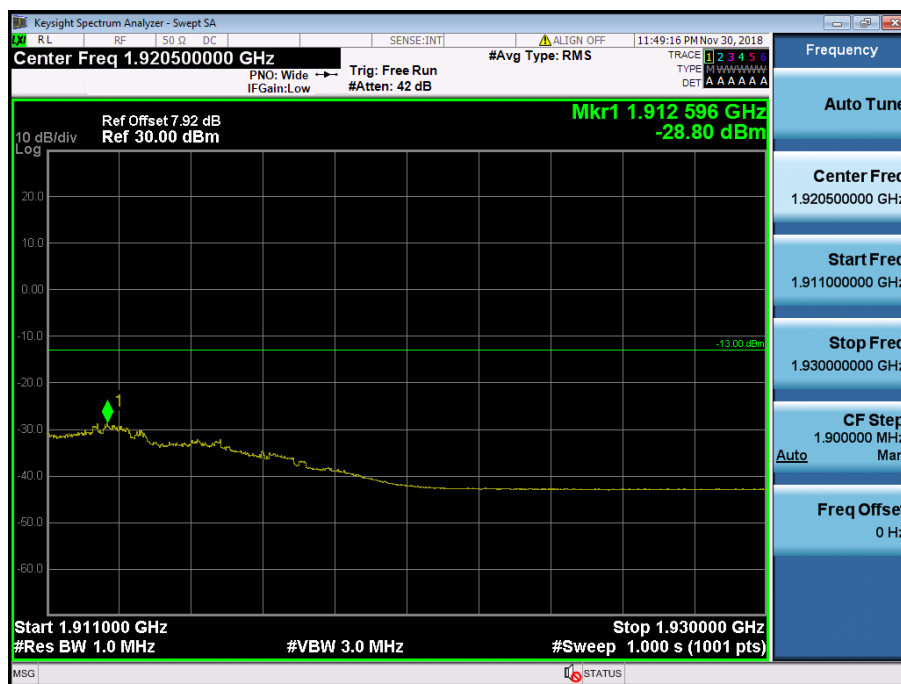
LTE Band 2 / 20MHz / QPSK - RB Size/Offset (50/50)
