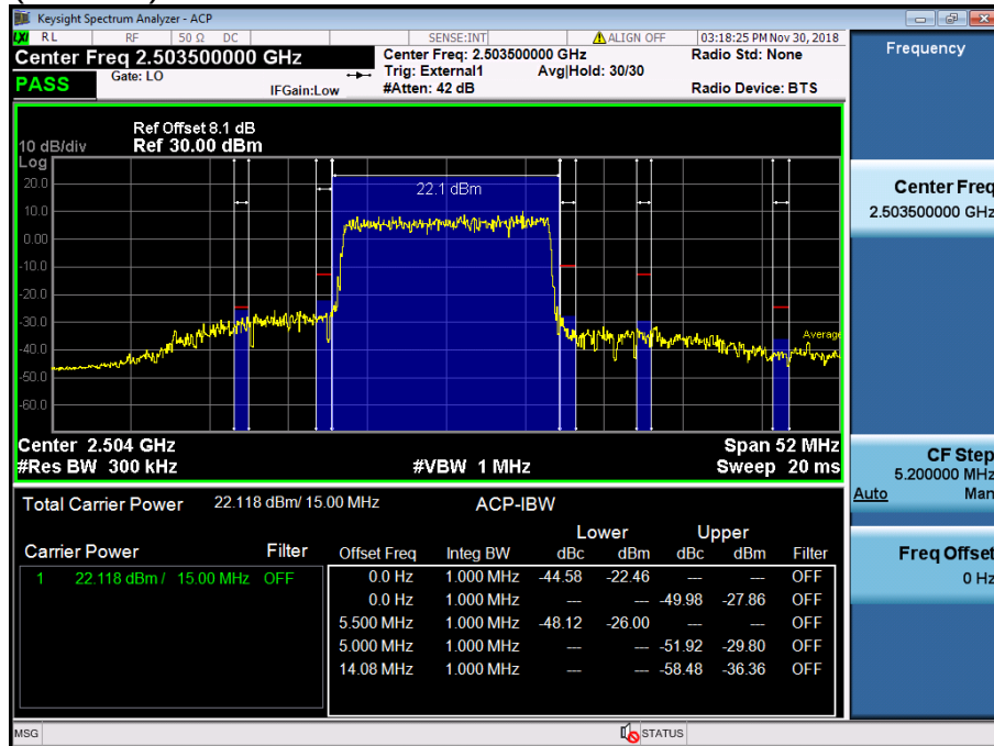
LTE Band 41 / 15MHz / QPSK - RB Size/Offset (75/0)
