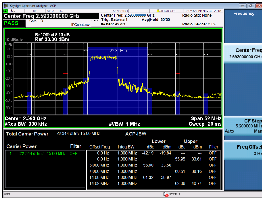
LTE Band 41 / 15MHz / QPSK - RB Size/Offset (36/0)
