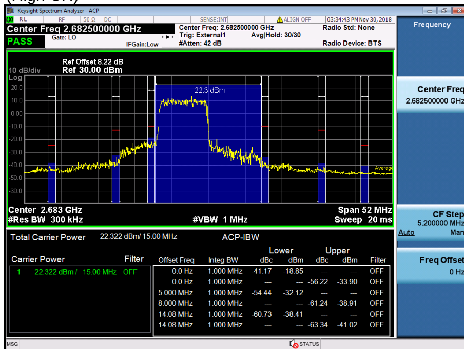
LTE Band 41 / 15MHz / QPSK - RB Size/Offset (36/0)
