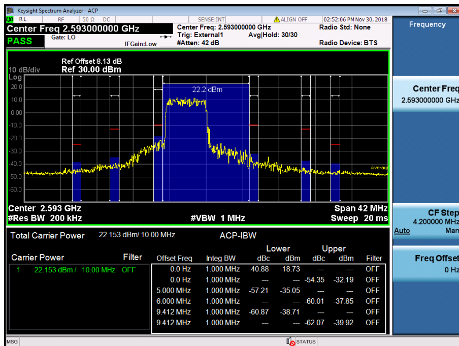
LTE Band 41 / 10MHz / QPSK - RB Size/Offset (25/0)
