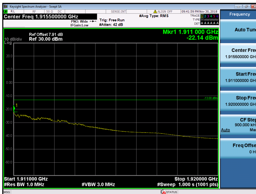
LTE Band 2 / 10MHz / QPSK- RB Size/Offset (25/25)
