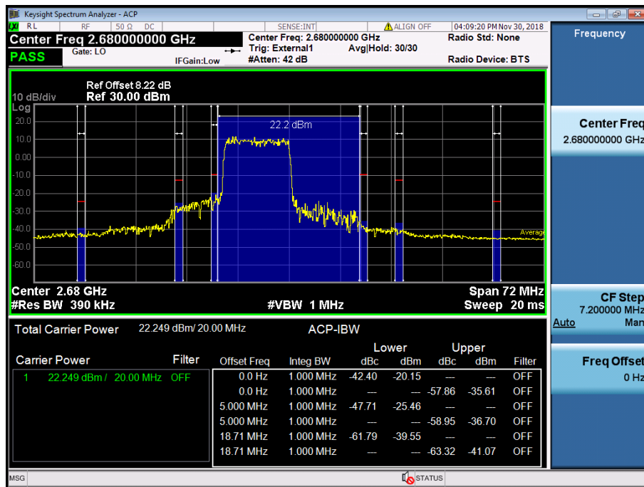
LTE Band 41 / 20MHz / QPSK - RB Size/Offset (50/0)
