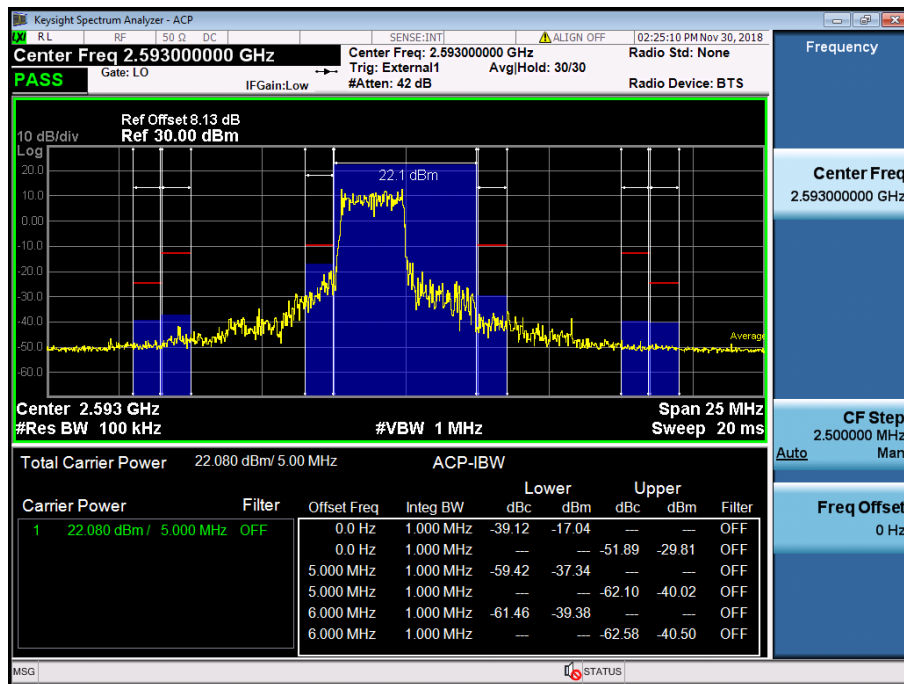
LTE Band 41 / 5MHz / QPSK - RB Size/Offset (12/0)
