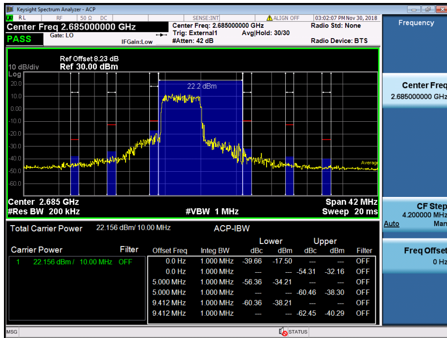
LTE Band 41 / 10MHz / QPSK - RB Size/Offset (25/0)
