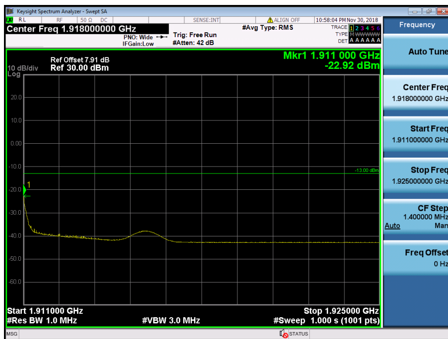
LTE Band 2 / 15MHz / QPSK - RB Size/Offset (1/74)
