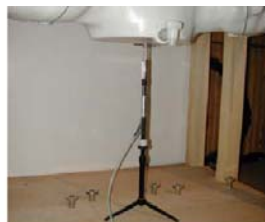
Figure 11.1 Dipole Verification Test Setup Diagram & Photo
