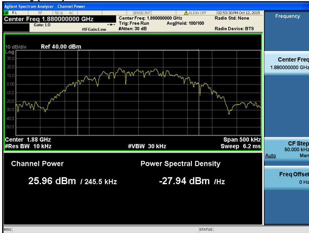
$$\text{PAR (dB)} = \text{P}_{\text{Pk}} (\text{dBm}) - \text{P}_{\text{Avg}} (\text{dBm}) = 29.86 \text{ dBm} - 25.96 \text{ dBm} = 3.90 \text{ dB}$$
