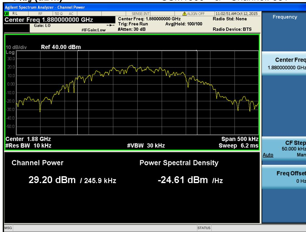
$$\text{PAPR (dB)} = \text{P}_{\text{pk}} (\text{dBm}) - \text{P}_{\text{avg}} (\text{dBm}) = 29.31 \text{ dBm} - 29.20 \text{ dBm} = 0.11 \text{ dB}$$
