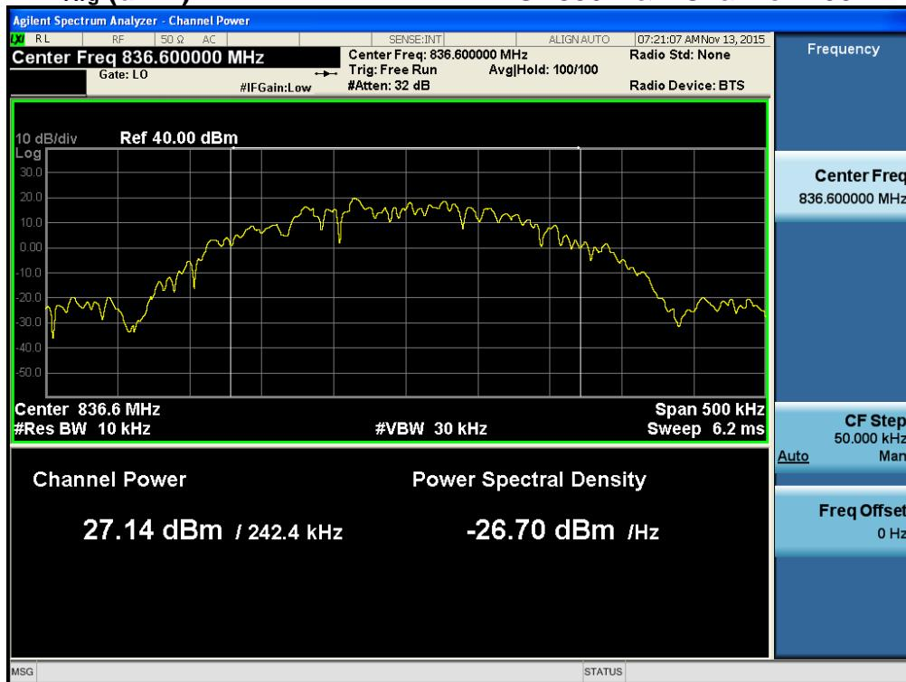
$$\text{PAR (dB)} = \text{P}_{\text{Pk}} \text{ (dBm)} - \text{P}_{\text{Avg}} \text{ (dBm)} = 31.96 \text{ dBm} - 27.14 \text{ dBm} = 4.82 \text{ dB}$$
