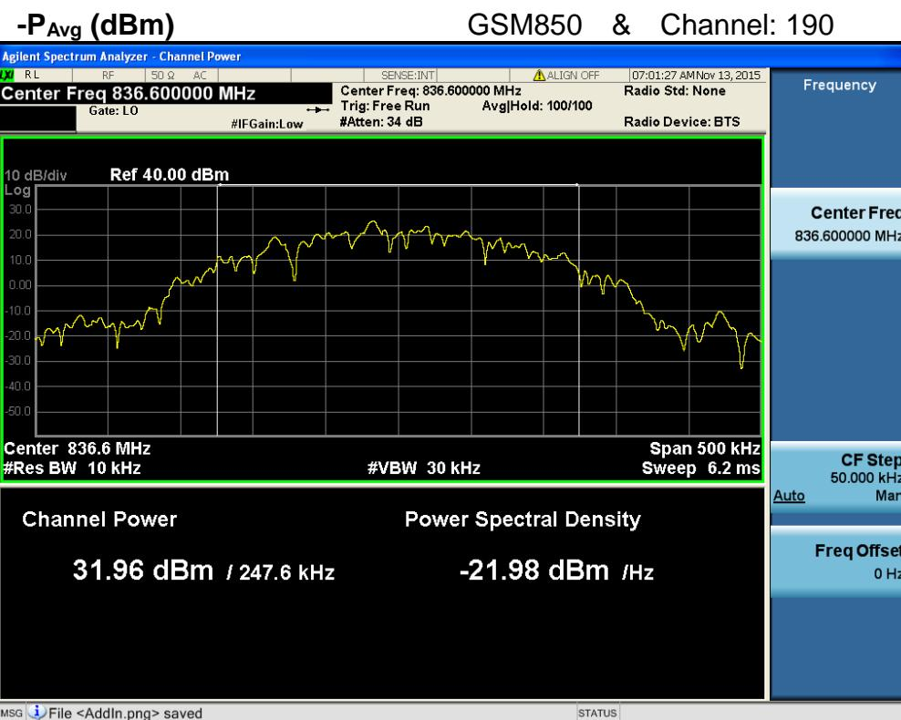
$$\text{PAPR (dB)} = \text{P}_{\text{Pk}} (\text{dBm}) - \text{P}_{\text{Avg}} (\text{dBm}) = 32.10 \text{ dBm} - 31.96 \text{ dBm} = 0.14 \text{ dB}$$
