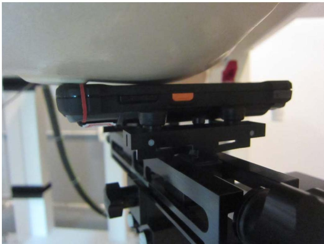
**■ Test Setup Photo (Head SAR Test Photo)**
