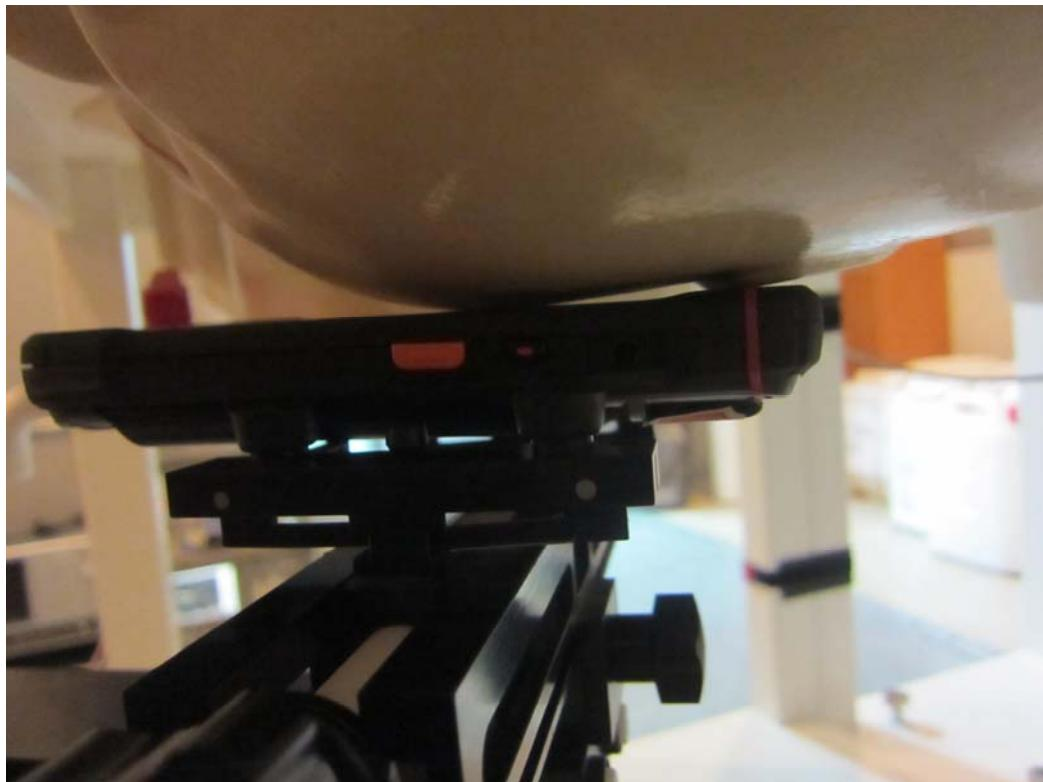
**■ Test Setup Photo (Body-Worn SAR Test Photo)**
