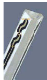
Figure 3.3 Probe Thick-Film Technique
