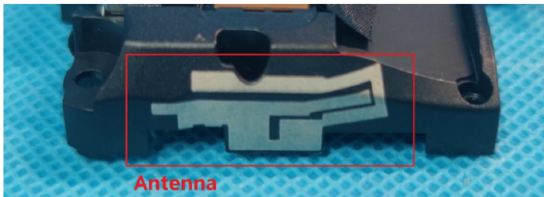
Picture 3 TOP antenna photo
