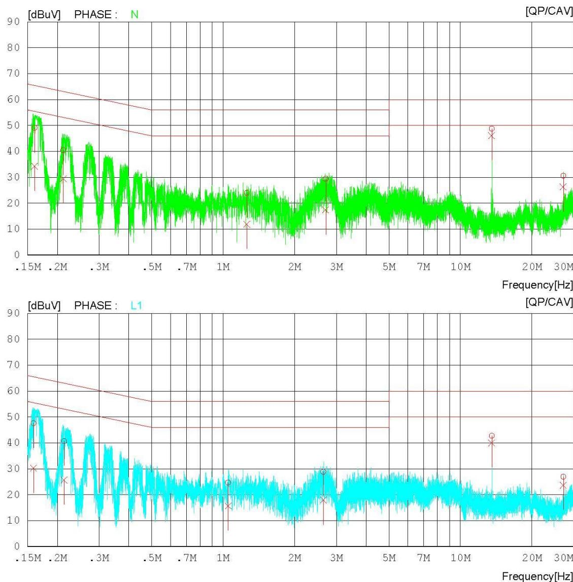
**Measurement Data****Results of Conducted Emission**
