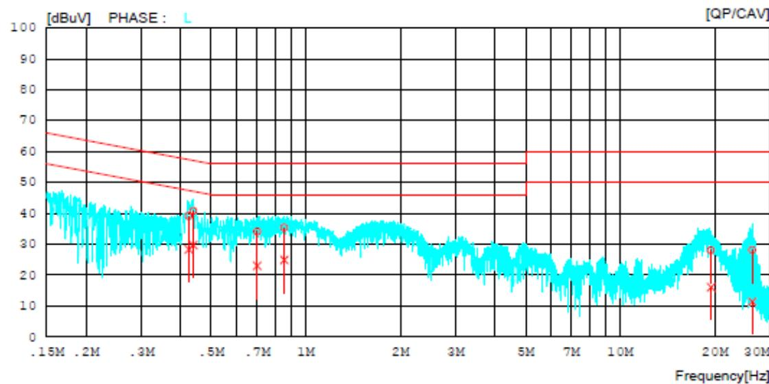
**AC Power-Line Conducted Emissions (List)****Results of Conducted Emission**
