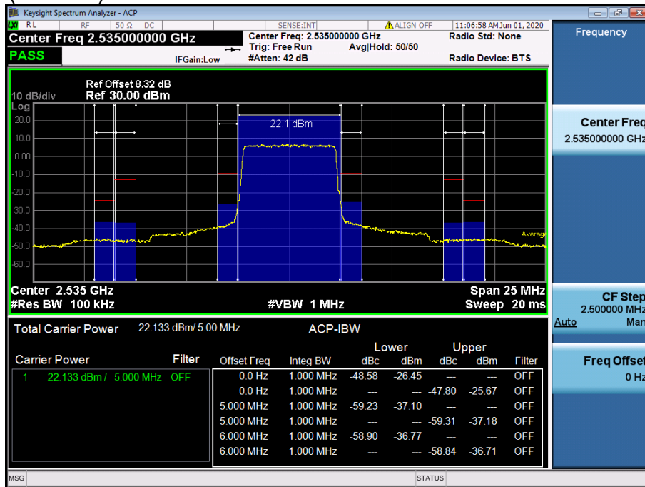
LTE Band 7 / 5 MHz / QPSK - RB Size/Offset (25/0)
