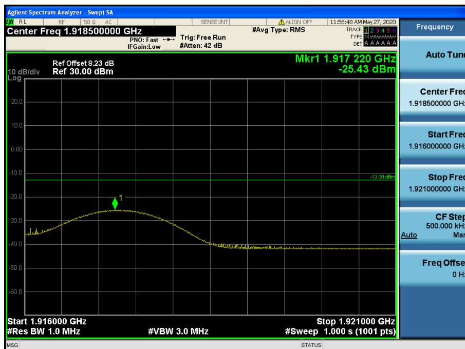
LTE Band 25 / 3 MHz / QPSK - RB Size/Offset (1/0)
