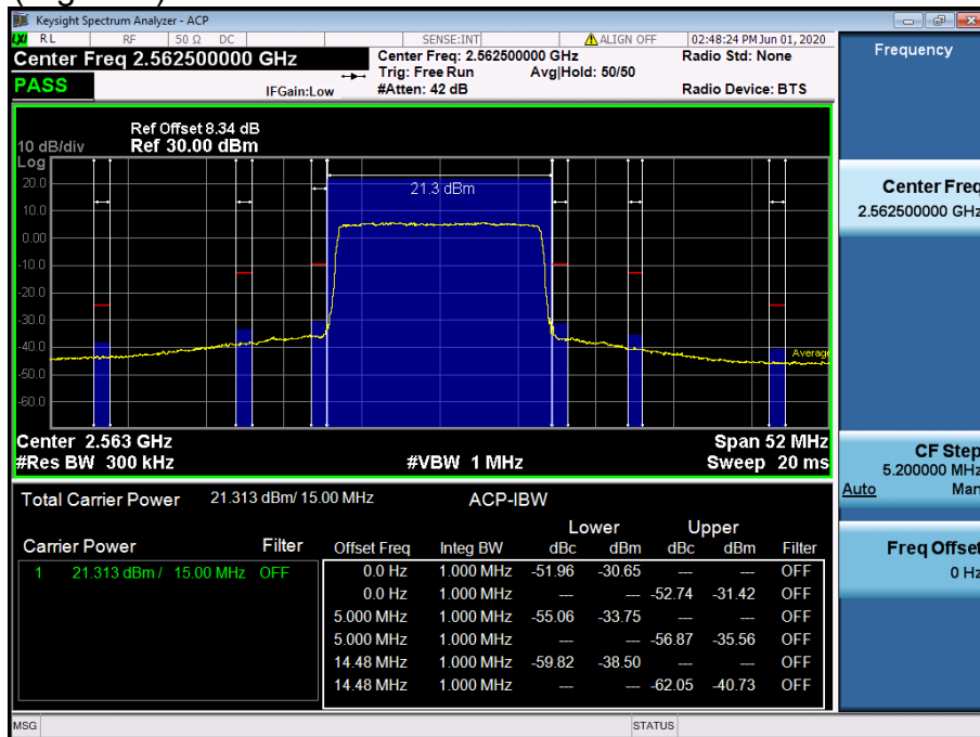
LTE Band 7 / 15 MHz / 16QAM - RB Size/Offset (75/0)
