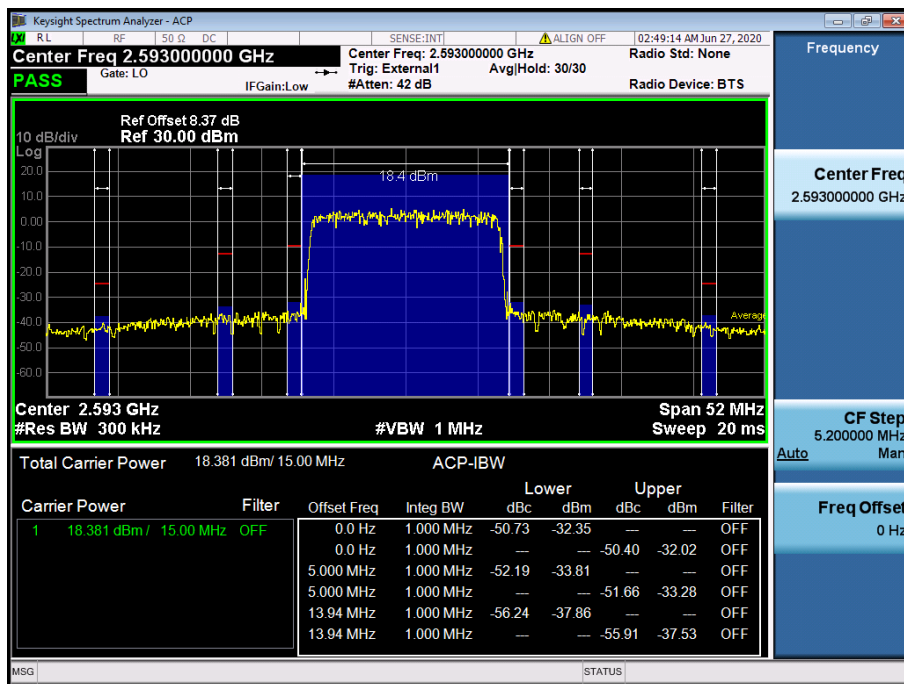
LTE Band 41 / 15 MHz / 16QAM - RB Size/Offset (75/0)
