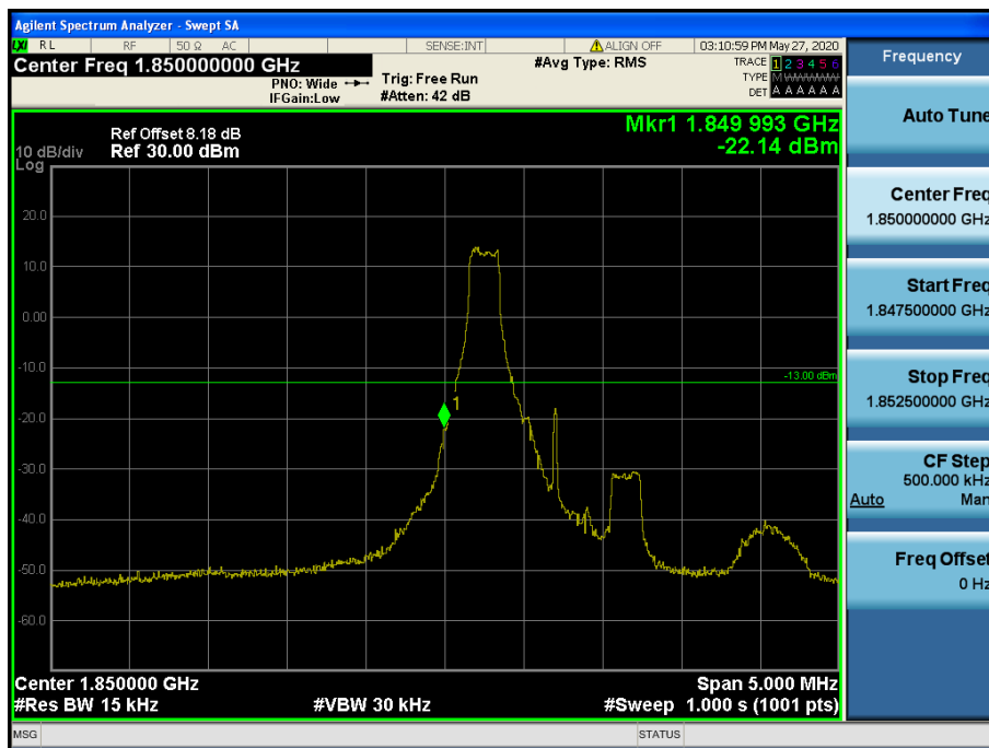
LTE Band 25 / 1.4 MHz / 16QAM - RB Size/Offset (1/0)
