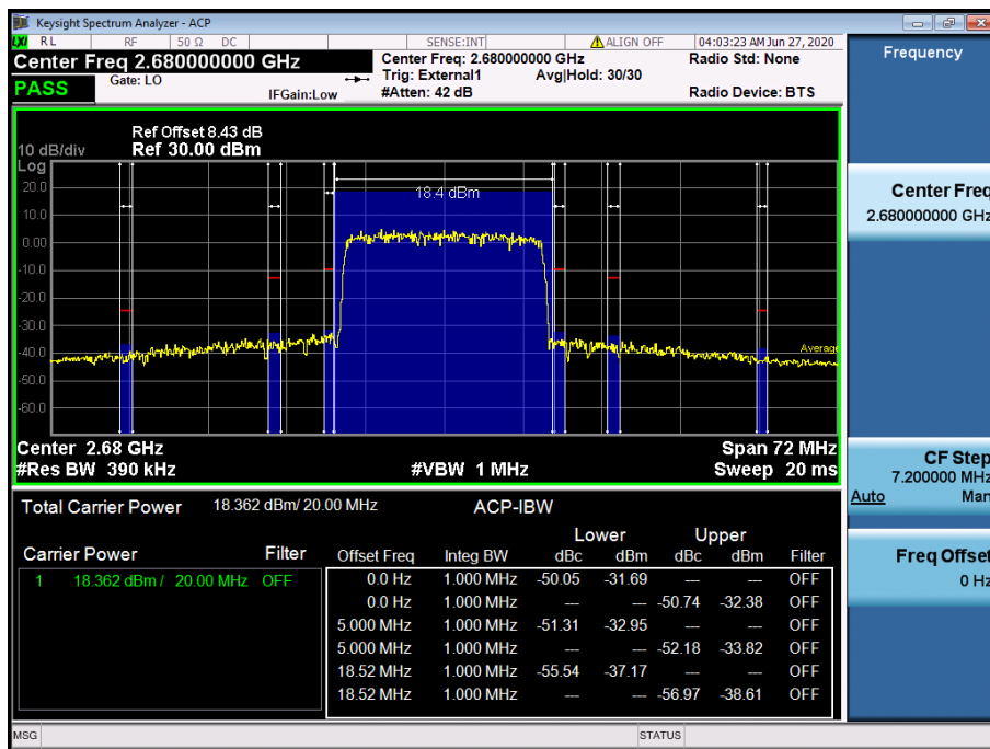
LTE Band 41 / 20 MHz / 16QAM - RB Size/Offset (100/0)
