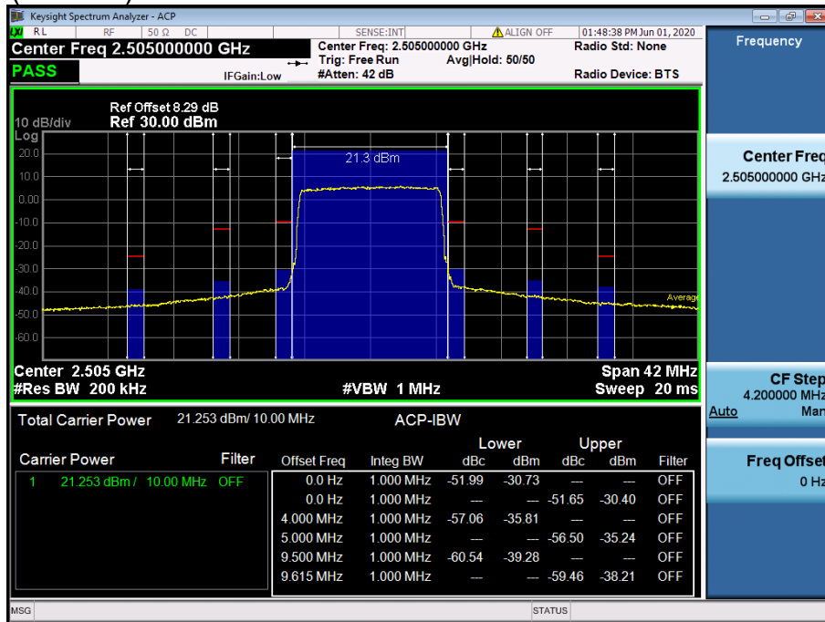
LTE Band 7 / 10 MHz / 16QAM - RB Size/Offset (50/0)
