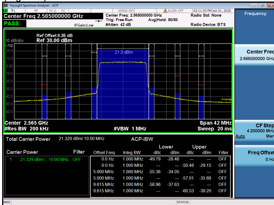
LTE Band 7 / 10 MHz / 16QAM - RB Size/Offset (50/0)
