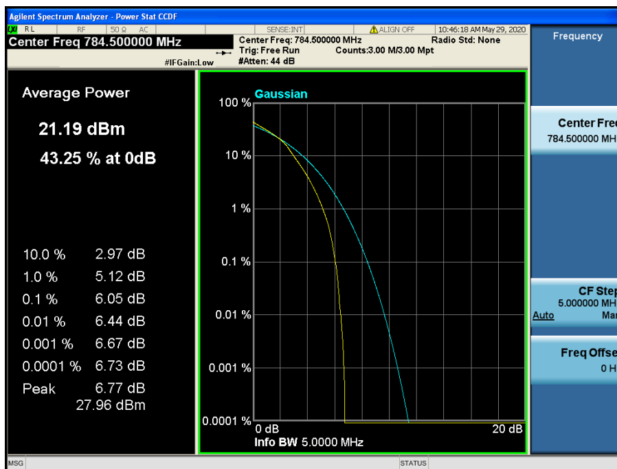
LTE Band 13 / 5 MHz / 16QAM - RB Size 25
