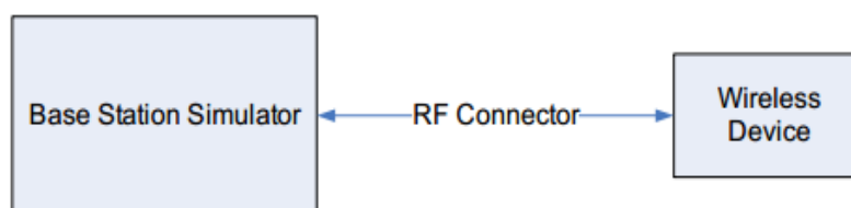
Figure 10.2 Power Measurement Setup
