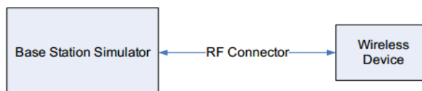
Figure 10.1 Power Measurement Setup
