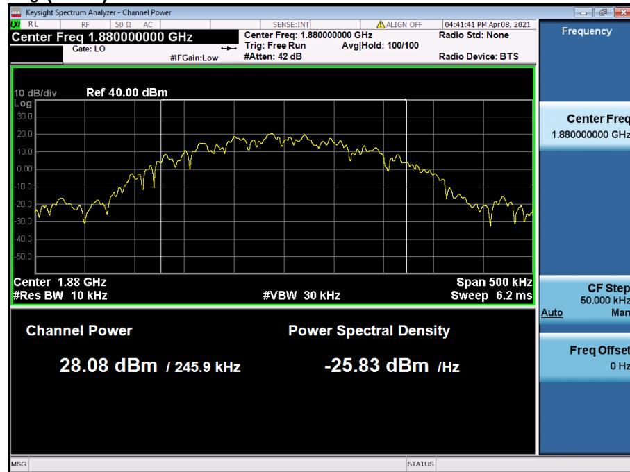
$$\text{PAPR (dB)} = \text{P}_{\text{Pk}} (\text{dBm}) - \text{P}_{\text{Avg}} (\text{dBm}) = 28.23 \text{ dBm} - 28.08 \text{ dBm} = 0.15 \text{ dB}$$
