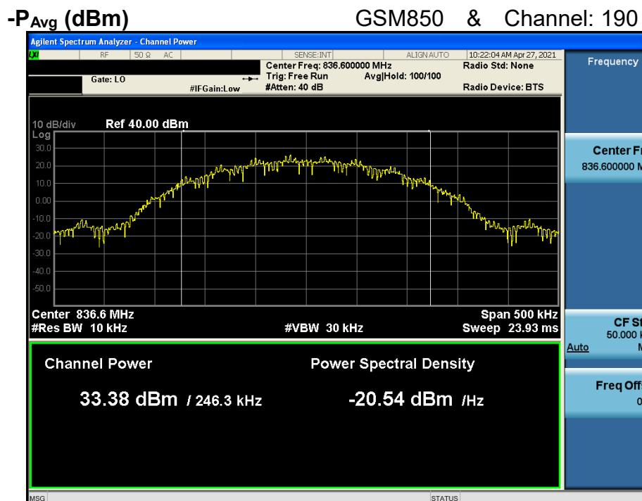
$$\text{PAPR (dB)} = \text{P}_{\text{Pk}} (\text{dBm}) - \text{P}_{\text{Avg}} (\text{dBm}) = 33.58 \text{ dBm} - 33.38 \text{ dBm} = 0.20 \text{ dB}$$
