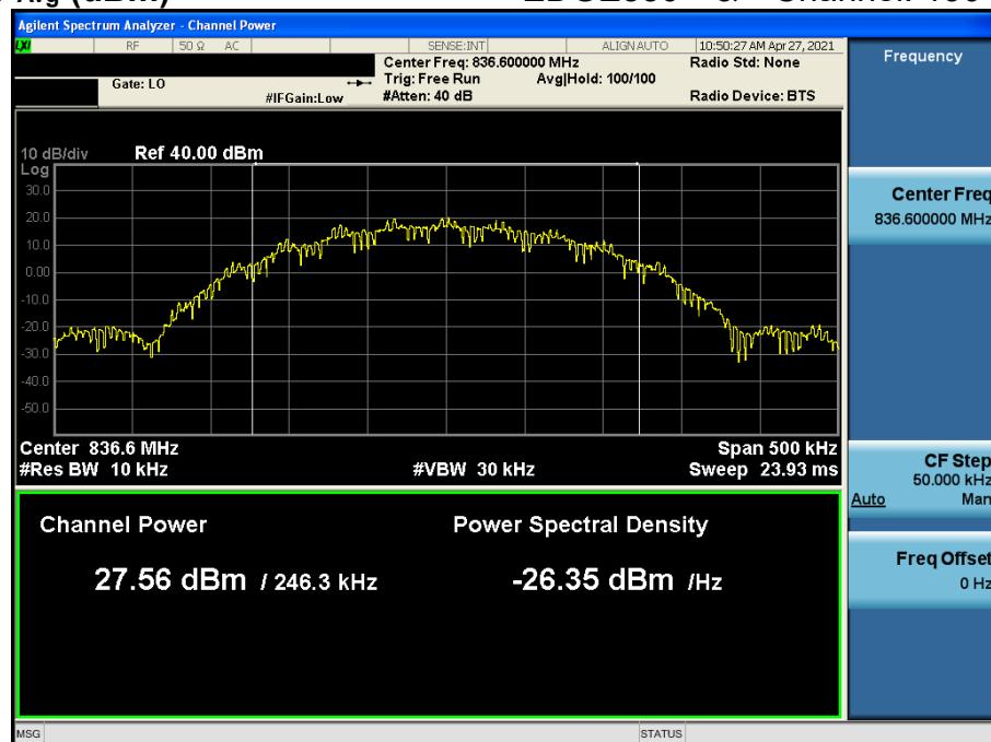
$$\text{PAPR (dB)} = \text{P}_{\text{Pk}} \text{ (dBm)} - \text{P}_{\text{Avg}} \text{ (dBm)} = 31.034 \text{ dBm} - 27.560 \text{ dBm} = 3.474 \text{ dB}$$
