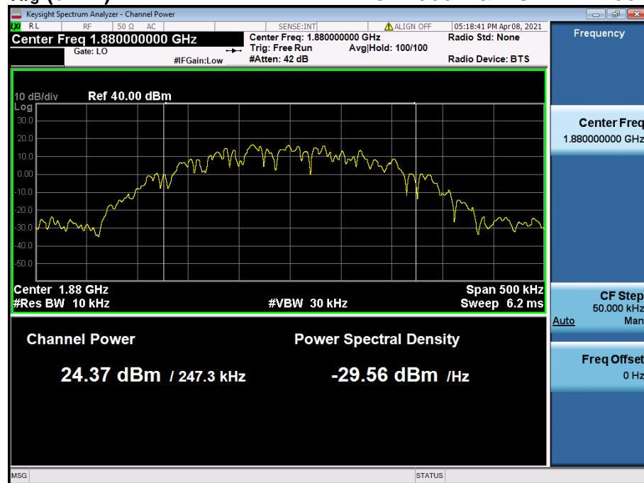
$$\text{PAPR (dB)} = \text{P}_{\text{Pk}} (\text{dBm}) - \text{P}_{\text{Avg}} (\text{dBm}) = 27.34 \text{ dBm} - 24.37 \text{ dBm} = 2.97 \text{ dB}$$
