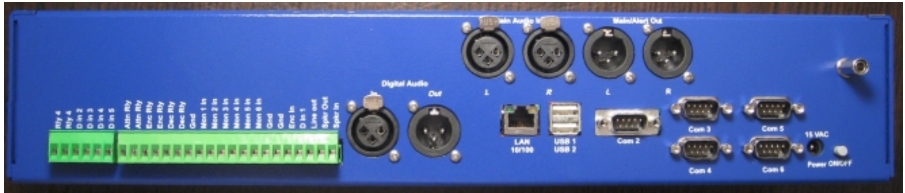
Exterior Back. Note: In the final product, “15 VAC” is replaced with “19 VDC”.
