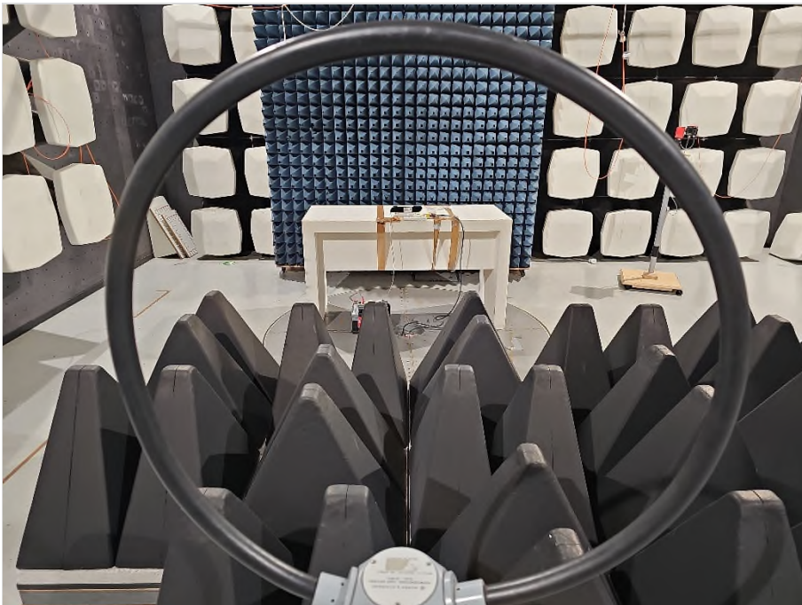
Photograph 4: EUT test setup in the anechoic chamber, overview_EUT elevation 0°
