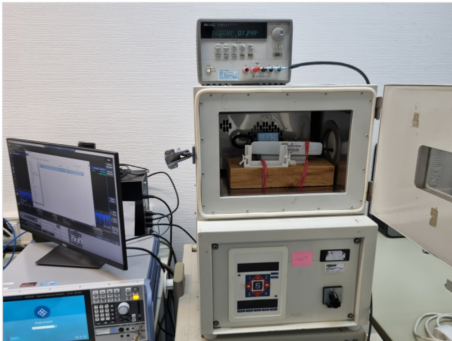
Photograph 7: EUT setup in the climatic chamber for test under extreme conditions, overview, EUT in TX mode
