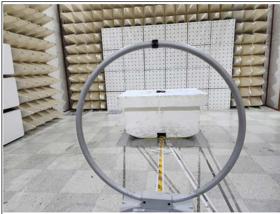
**3. Photo of Radiated Spurious Emission Test (30 MHz ~ 1 000 MHz)**
