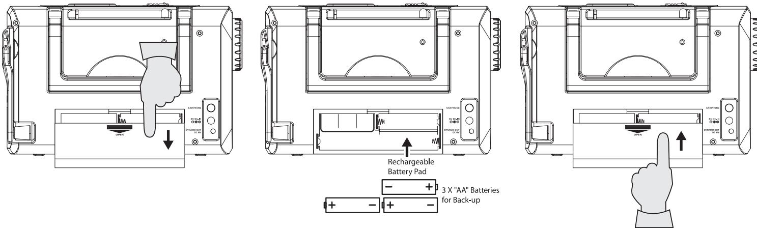
Replace the 3 "AA" batteries with new ones when the low battery indicator illuminates, the sound become unstable, or the clock display no longer functions.
