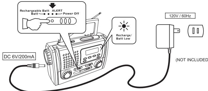
Note: Keep the AC Adaptor (Not Included) connected for about 12 hours to fully charge.
