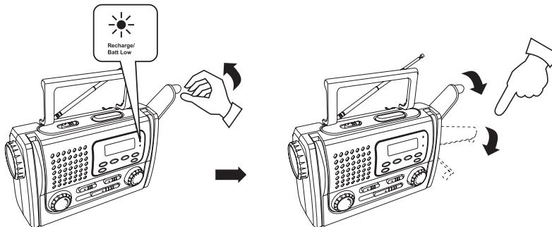
Note: Turn the Dynamo hand-crank clockwise at a moderate speed for about 1 minute. This will provide a 1/4 charge.
